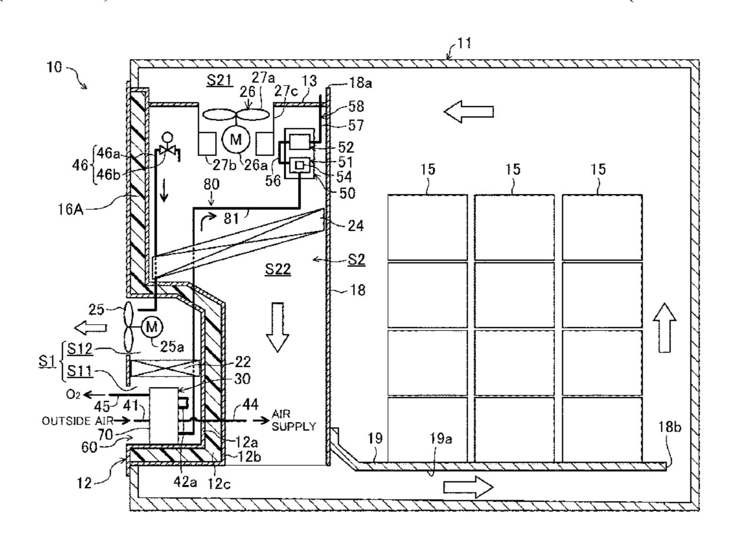
if a carbon dioxide concentration of the inside air is lowered to a critical concentration lower than a target carbon dioxide concentration, and restarts the gas supply operation if the carbon dioxide concentration of the inside air has reached a restart concentration higher than the target carbon dioxide concentration through breathing of the plants.
