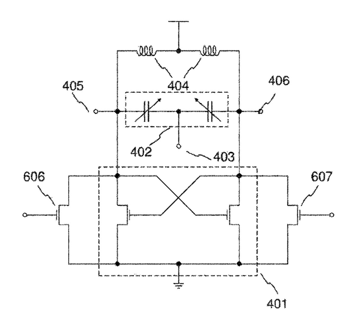
oscillation frequency of which is a function of a value of an inductive element of the LC oscillators and which are frequency-synchronized via a wiring, and forced by a control voltage to have a same oscillation frequency, is used as the receiver and/or the transmitter. A controller configured to control the assembly is connected, the assembly and the controller are configured to generate a magnetic field capable of deflecting a magnetization of the sample out of equilibrium.
