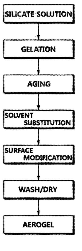
an amount such that an amount of magnesium ions is greater than 50 mol % based on a total mole of metal ions in the metal salt solution, and a metal oxide-silica composite aerogel having low tap density and high specific surface area prepared by the method.
