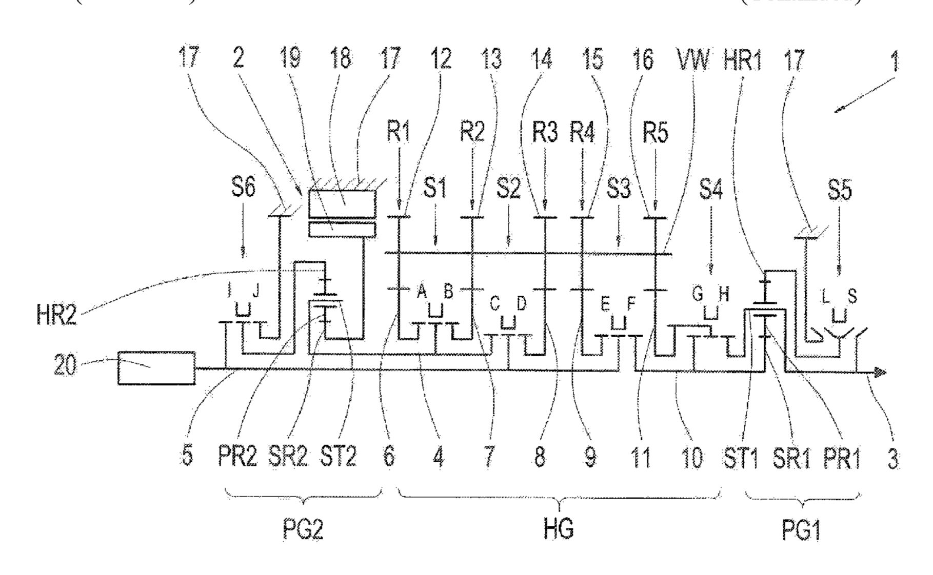
gear set (PG1) either to the output shaft or a housing. An electric machine is permanently connected to an element of gear set (PG2). If, while driving with a transmission gear engaged, the drive output brake is engaged for a full brake application, a shift element of the transmission is first relieved by the electric machine and/or a brake assigned to one of the input shafts and then subsequently disengaged to decouple the combustion engine from the drive output.
