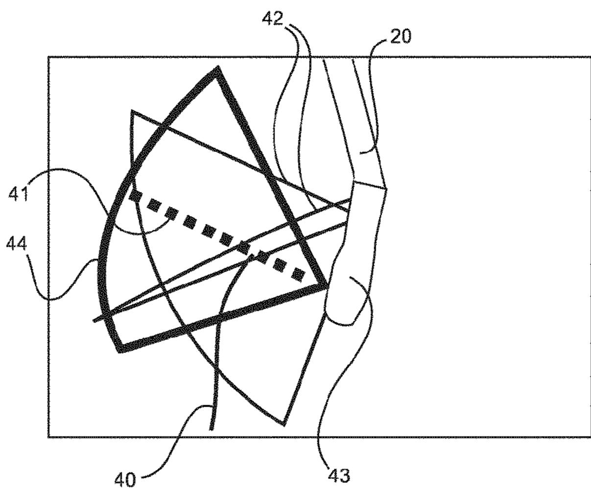
processing unit (12) is configured to determine a plane (41) orthogonal to a tangent of the centerline as viewing plane. The processing unit (12) is configured to calculate an imaging plane and an imaging orientation of the TEE probe (20) to lie approximately in the viewing plane. The processing unit (12) is configured to provide the calculated data as guidance data.
