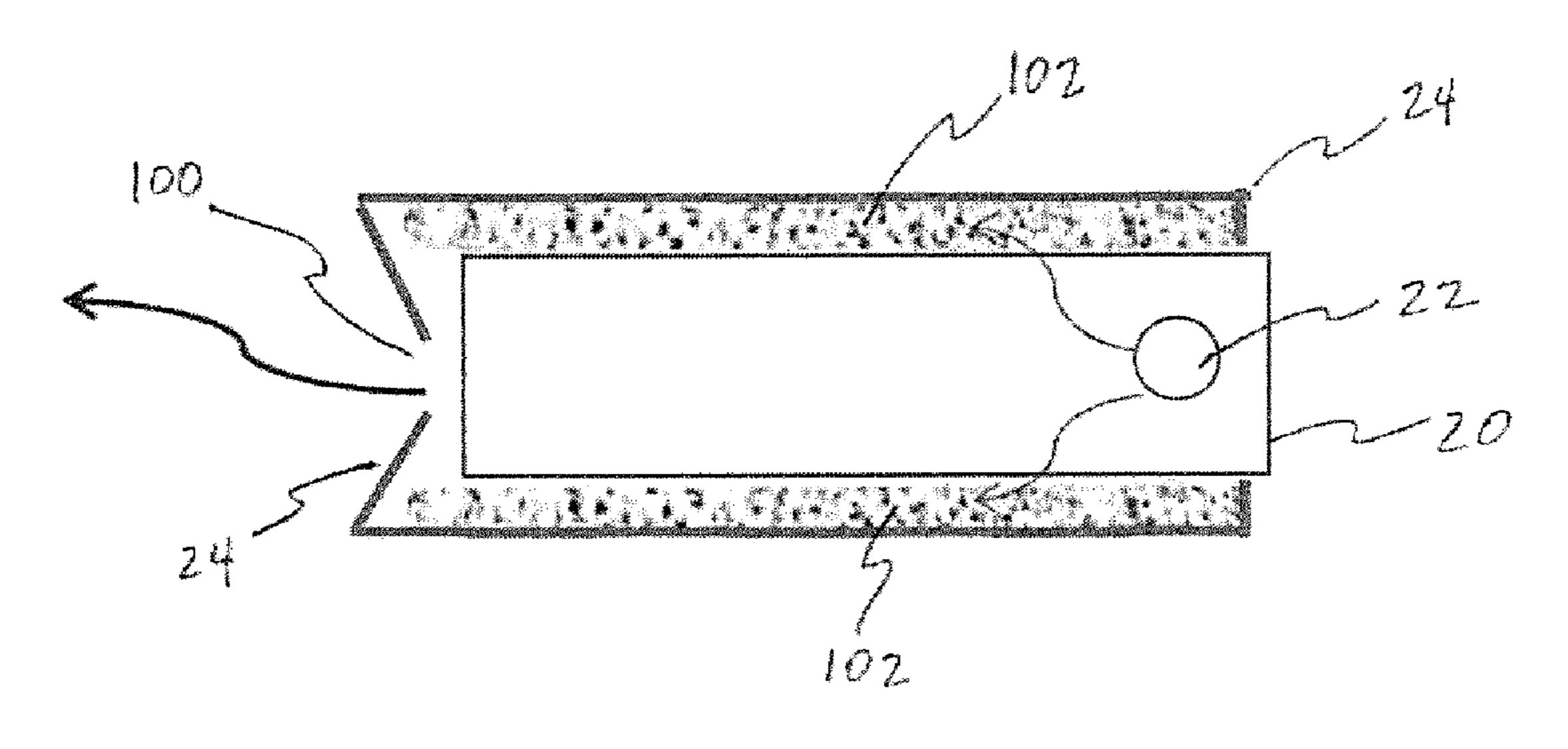
the inflator via the inflator discharge port; and a permeable gas diffuser element disposed in or adjacent to the tube, the diffuser element being configured to receive gas from the inflator via the inner tube.
