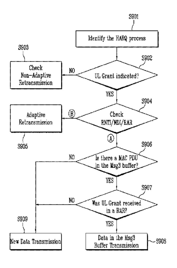
Msg3 buffer when receiving the UL Grant signal on the specific message and the specific message is the random access response message.
