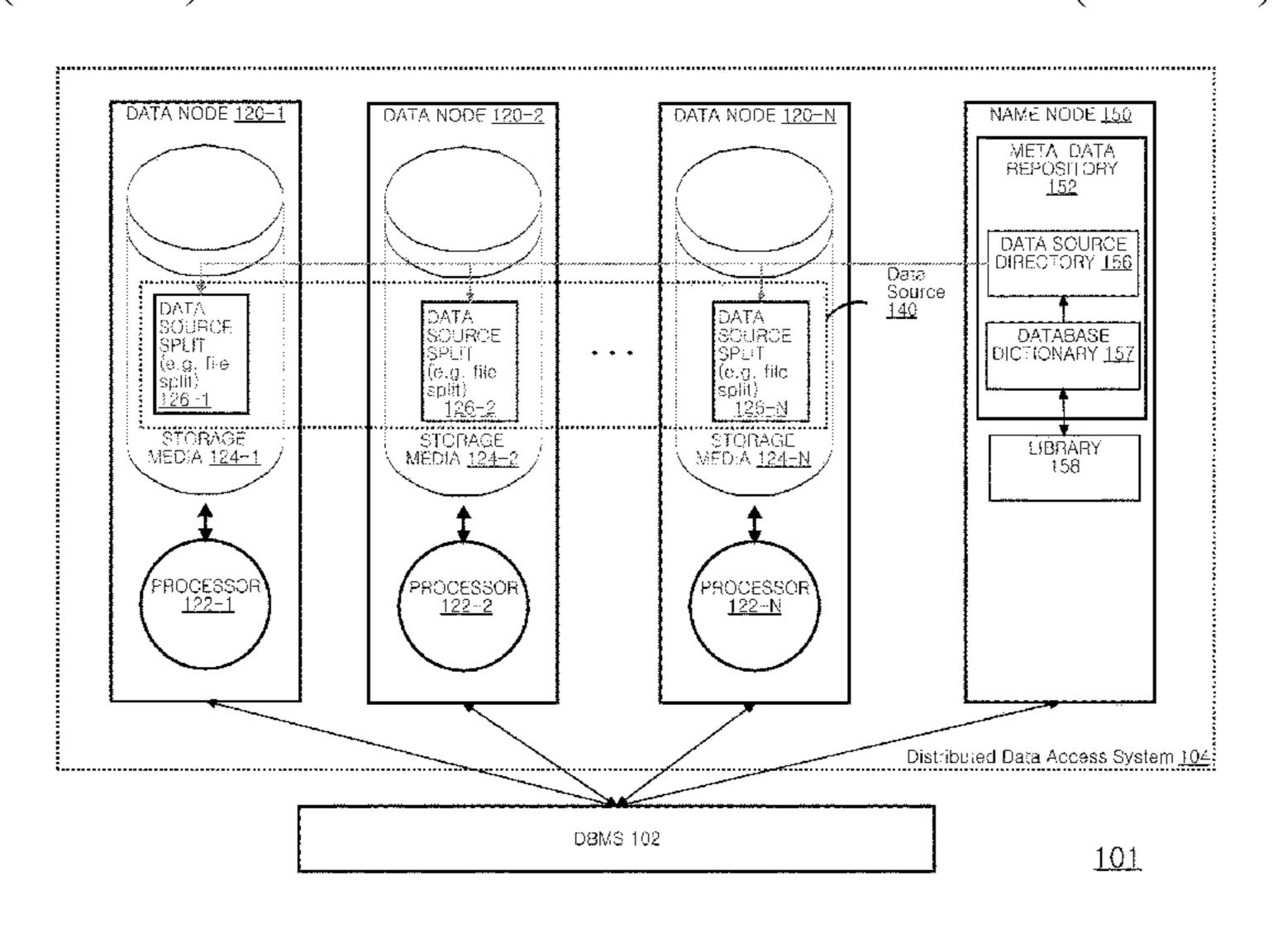
for each portion to the respective data node, requesting that the data node generate rows from data in the portion. The request may specify scanning criteria, specifying one or more columns to project and/or filter on, and code modules for the data node to execute to generate records.
