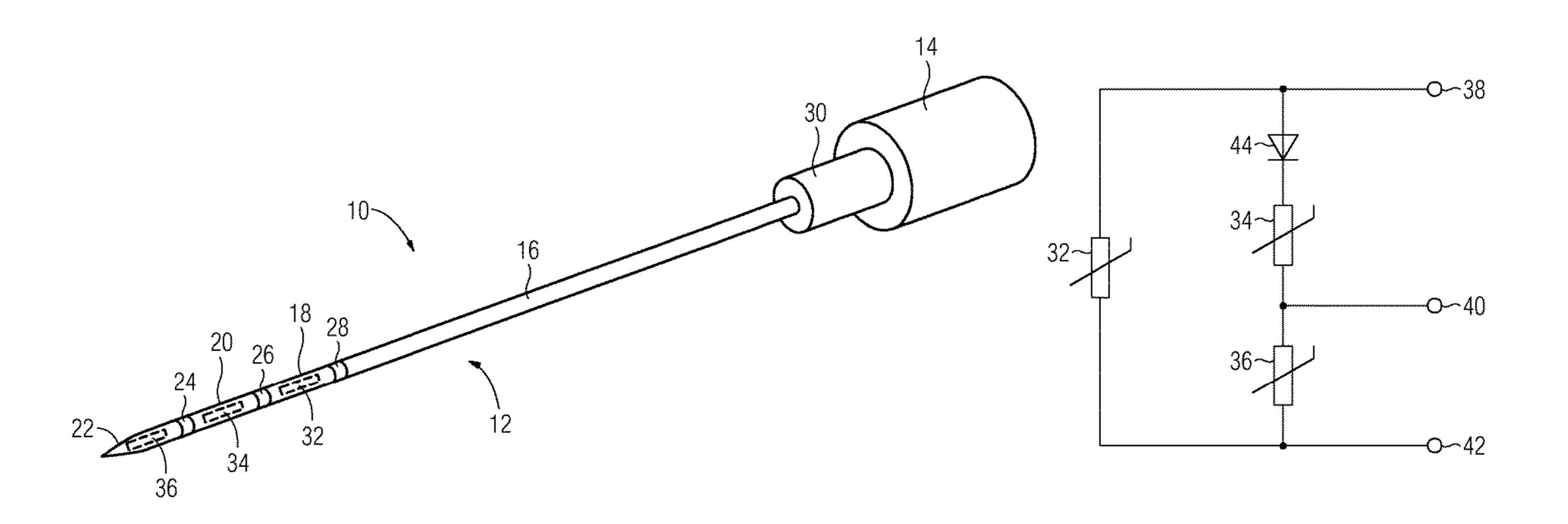
pipe section (18, 20) and/or inside the cone end (22). The food probe (10) comprises a connector (38, 40, 42) provided for an electric connection to a control unit. The connector comprises at least three connector elements (38, 40, 42) connected to the temperature sensors (32, 34, 36) according to the predetermined scheme. Further, the present invention relates to a method for controlling a cooking process.
