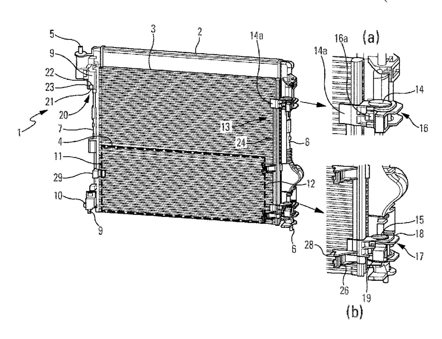
radiator (2) by means of a junction member (13) disposed between the main radiator (2) and at least one first auxiliary heat exchanger (3), The junction member (13) is principally formed of at least two shaft bearings (14, 15) attached to the first auxiliary heat exchanger (3) and nested inside respective open flanges (16, 17) formed on one of the lateral sides (7, 8) of the main radiator (2).
