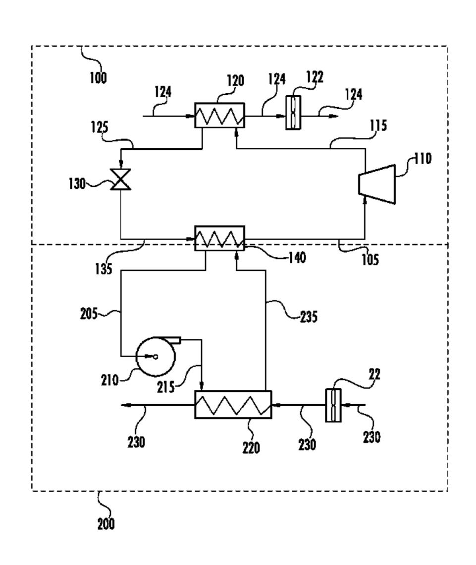
indoor, two phase heat transfer fluid circulation loop that transfers heat to the first loop through the heat exchanger evaporator condenser. The second loop includes the heat rejection side of the heat exchanger evaporator condenser, a liquid pump, and a heat exchanger evaporator, connected by conduit in a closed loop and having disposed therein a second heat transfer fluid that has an ASHRAE Class A toxicity rating and an ASHRAE Class 1 or 2L flammability rating.
