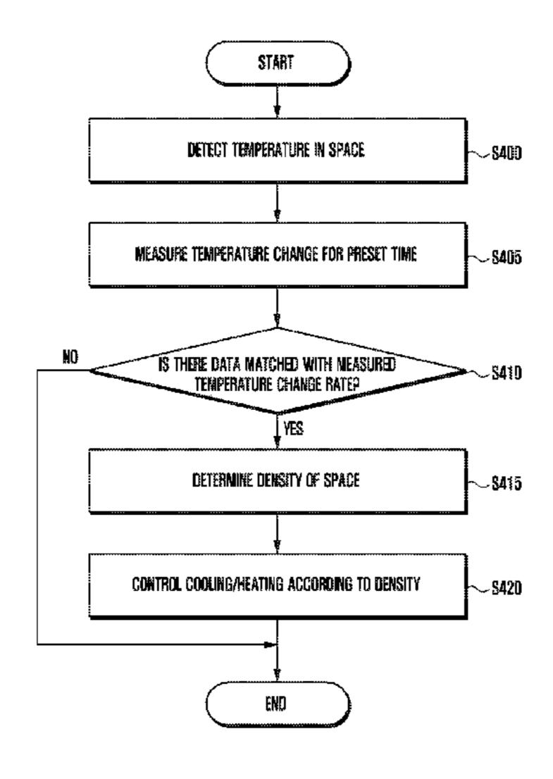
information on a location at which the temperature change is measured; and controlling air-conditioning according to the first density information.
