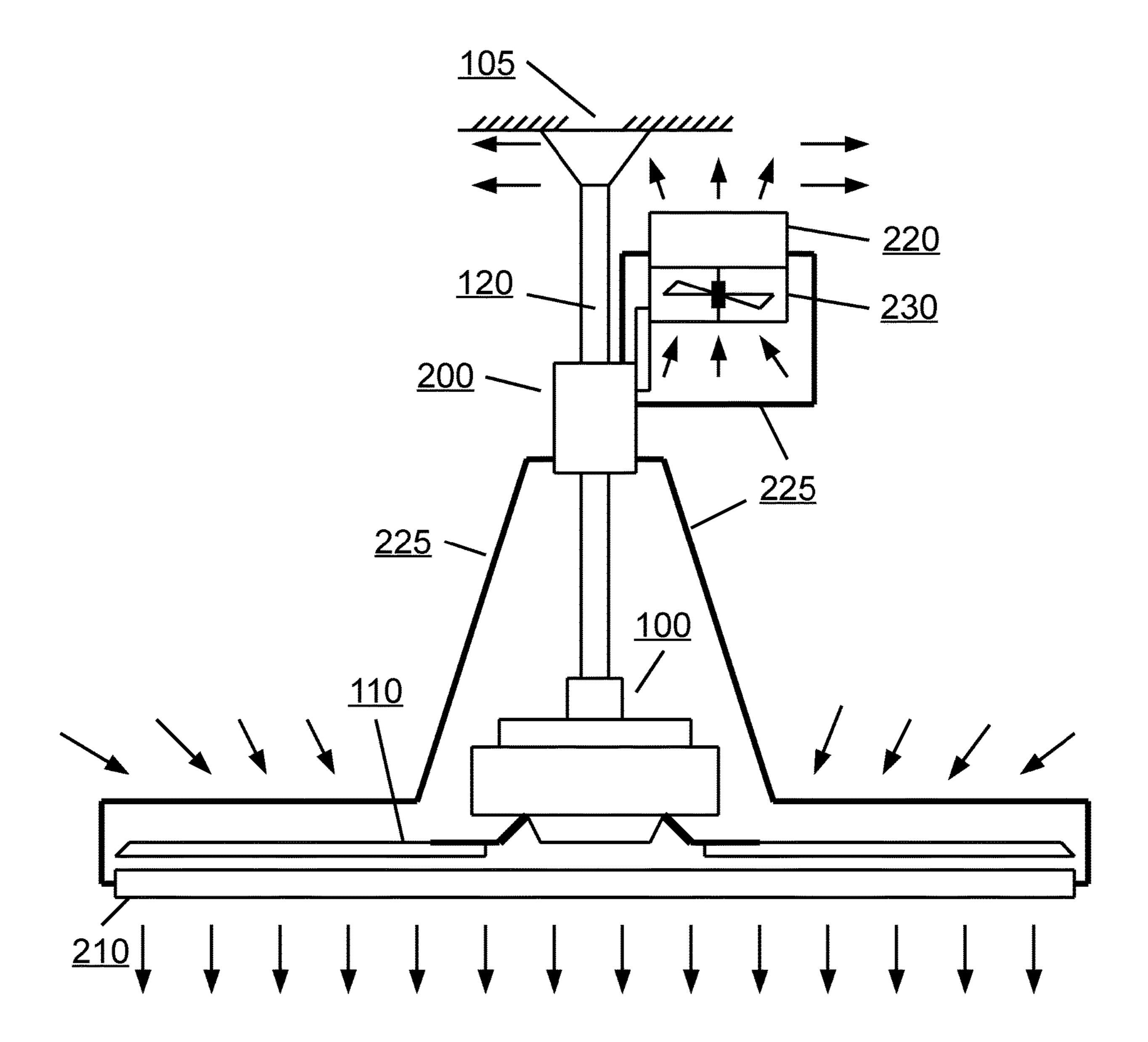
Schematic diagram of preferred embodiment of invention (Arrows show general direction of air flow)
