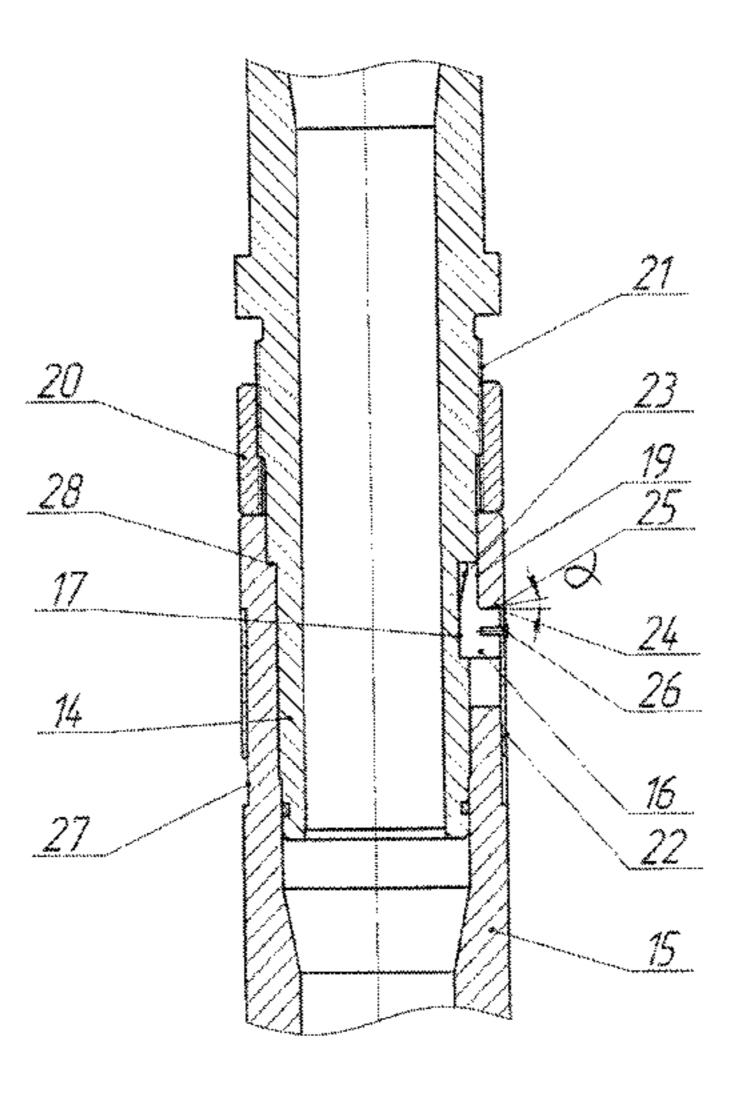
coupled housings each have the covering and the covered parts, and the covered part of one of the housings contains a blind rectangle groove, and the covering part of another housing has a through rectangle groove, and the grooves form a cavity having an embedded ring segment.
