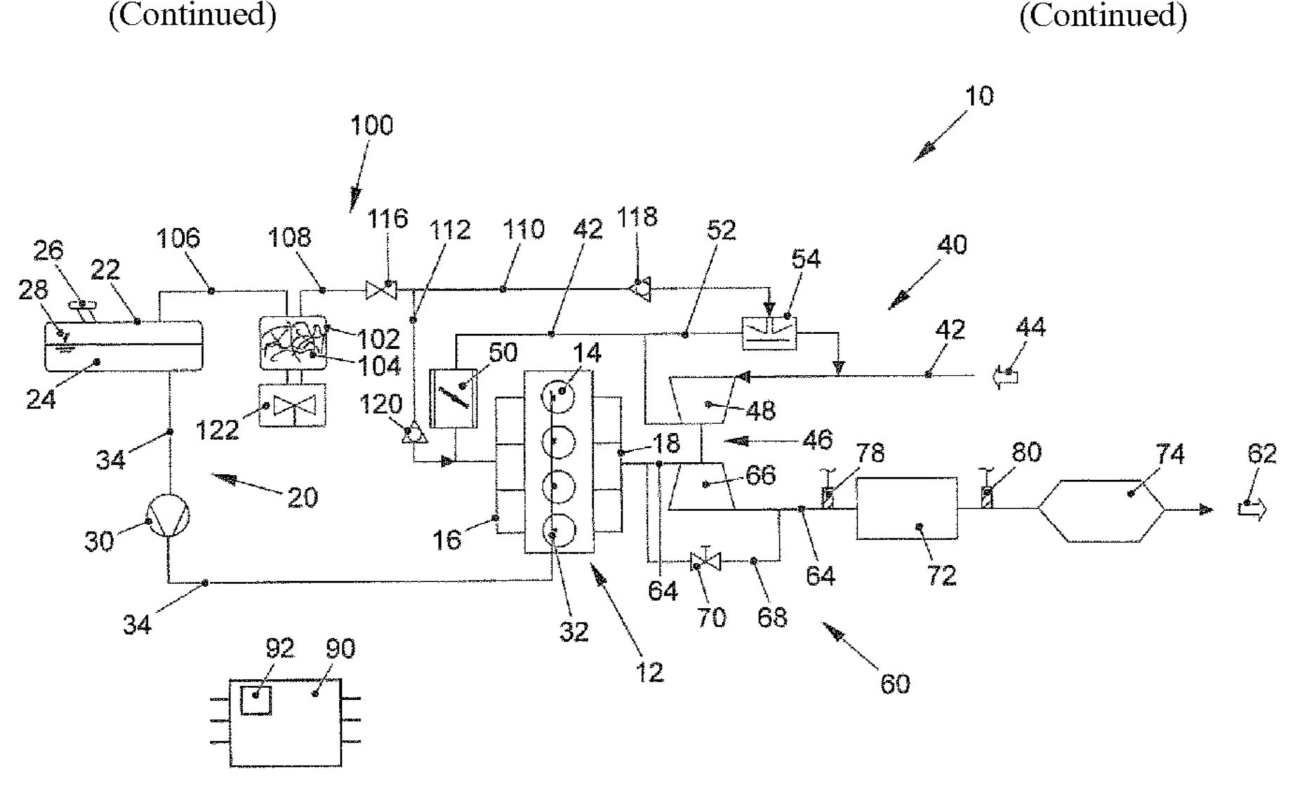
upstream of the particle filter (74). By means of an exothermic conversion of the fuel vapours (24) in the exhaust system (60) upstream of the particle filter (74), the exhaust-gas temperature (T) can be increased without the need for engine-internal measures for increasing the exhaust-gas temperature.
