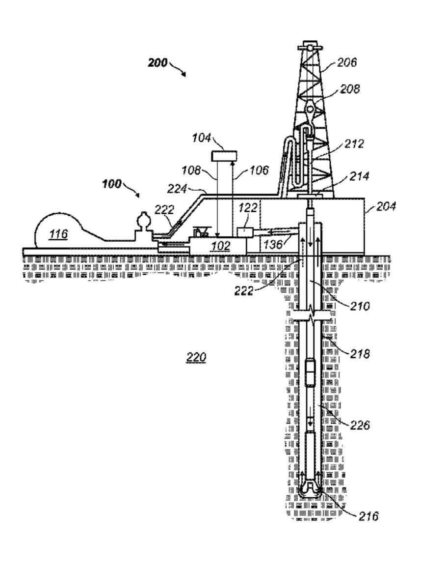
chemically tagged drilling fluid additive in a subterranean formation or a filter cake. An apparatus comprising: a vessel for holding a quantity of a drilling fluid a filter media; a mud sensor; a cake sensor; an outlet sensor; a data processing system coupled to the mud sensor, the cake sensor, and the outlet sensor.
