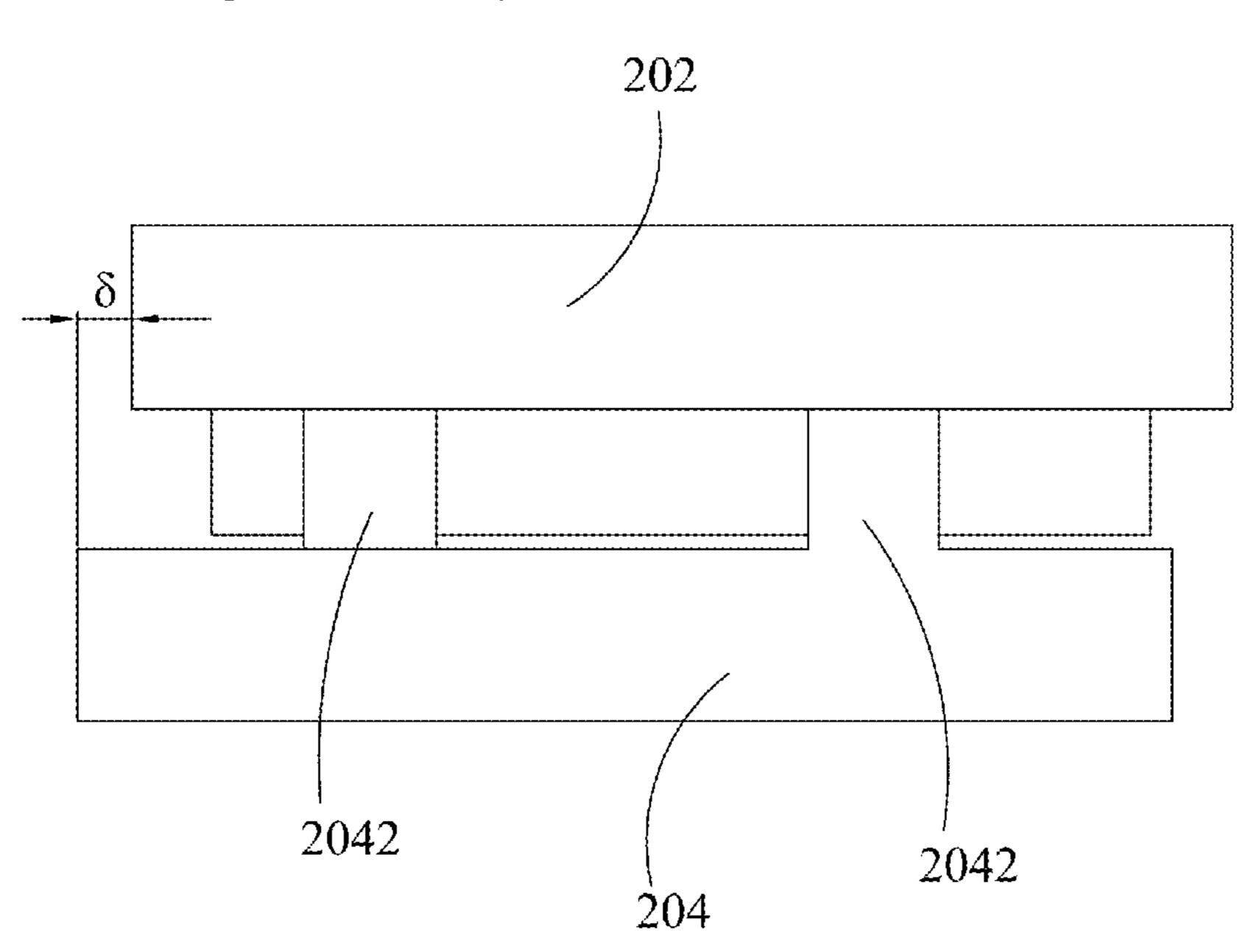
Provide a thermoforming mold, wherein the thermoforming mold comprises a lower mold and an upper mold arranged above the lower mold and matched therewith
