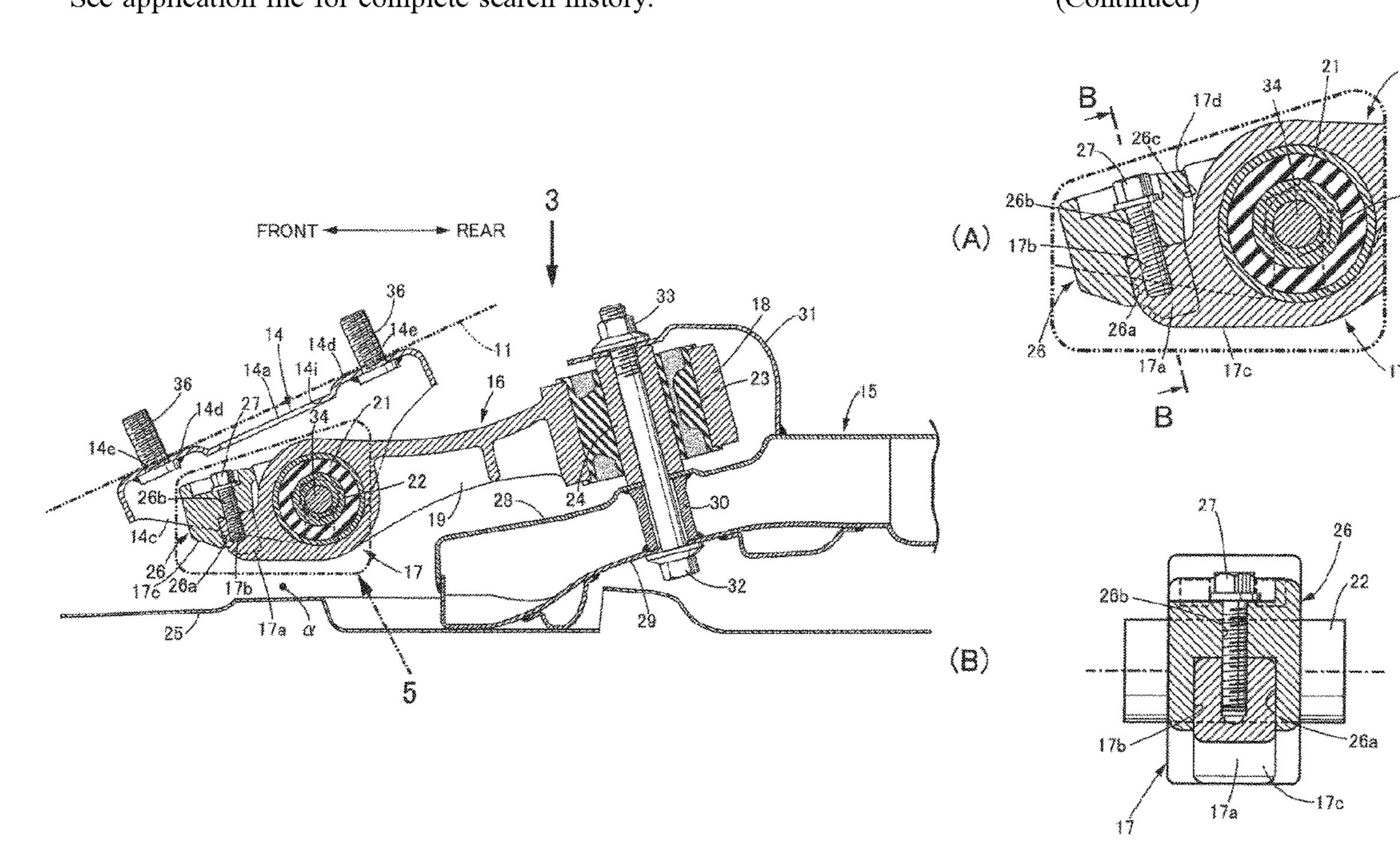
18 to each other. An outer circumferential face of the first end part 17 includes a projection part 17a which projects radially outward so as to extend away from the second end part 18, and a mounting part 17b to mount a mass body 26 is formed in the projection part 17a.
