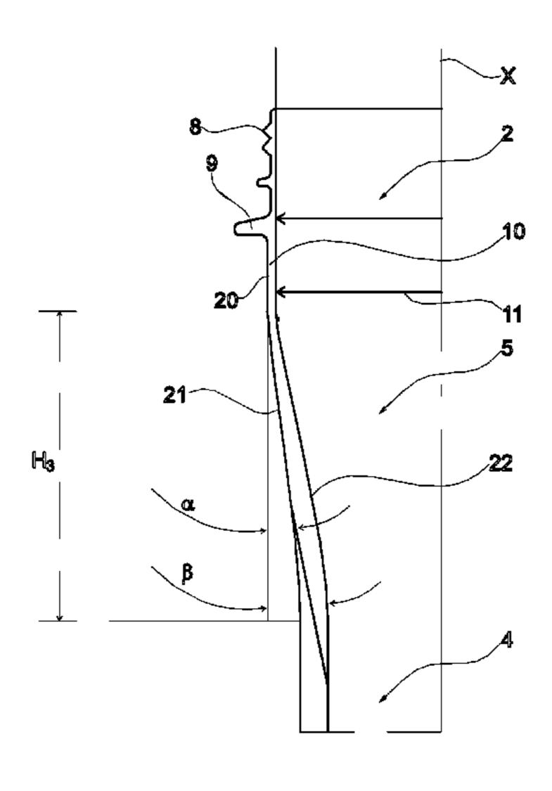
angle  $\alpha$  less accentuated than normal, max. 17°, which allows to make a preform with a thickness  $t_2$  of the wall thinner than 1.9 mm and a thinner inner diameter of the preform body in order to allow a lower stretch ratio starting from a larger preform to obtain the final bottle of predetermined capacity.
