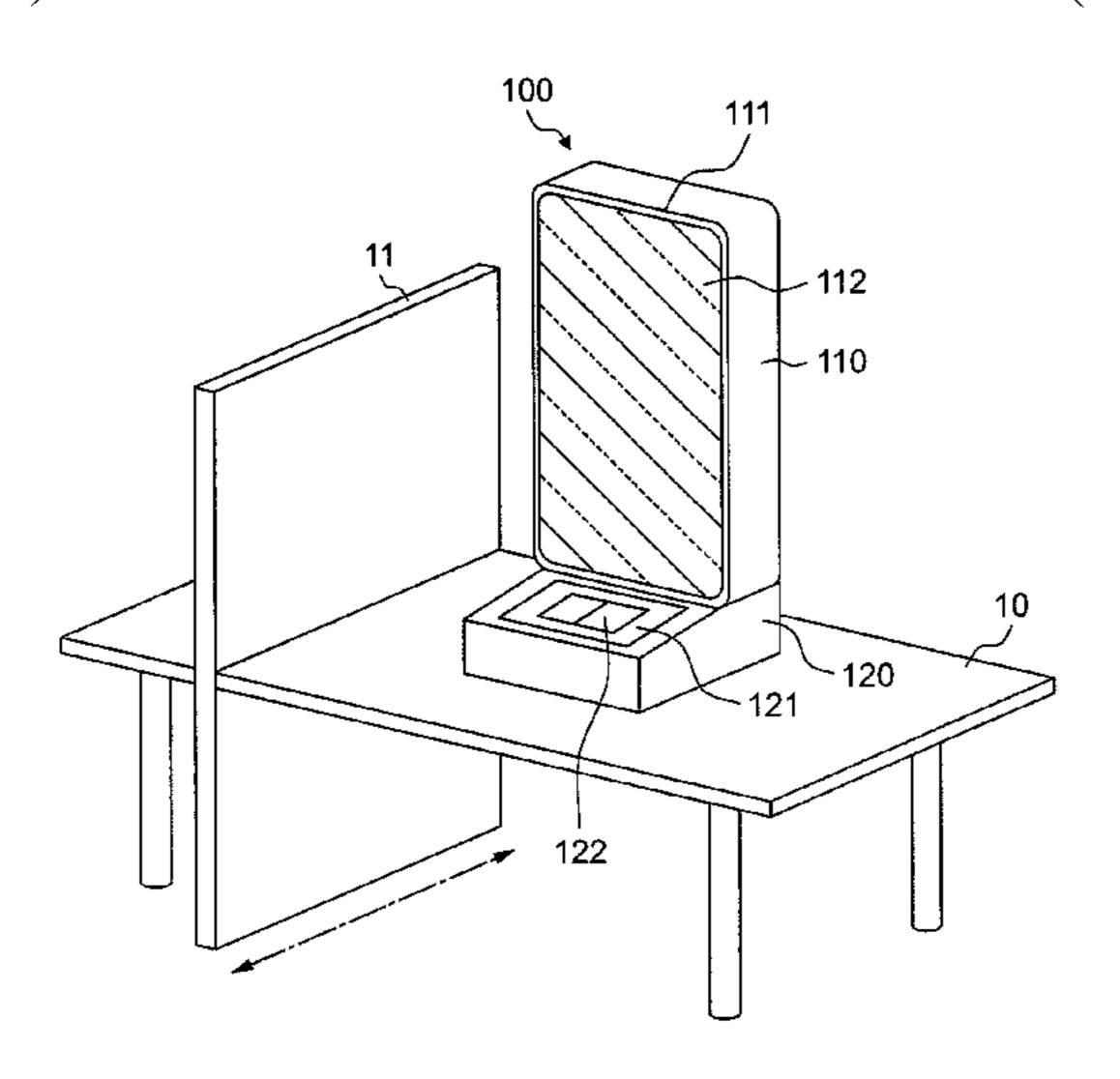
almost the same. As a result, it is possible to capture a face image suitable for collation by an imaging device while making a display suitable for collation by a display to a person in the front side of the half mirror.
