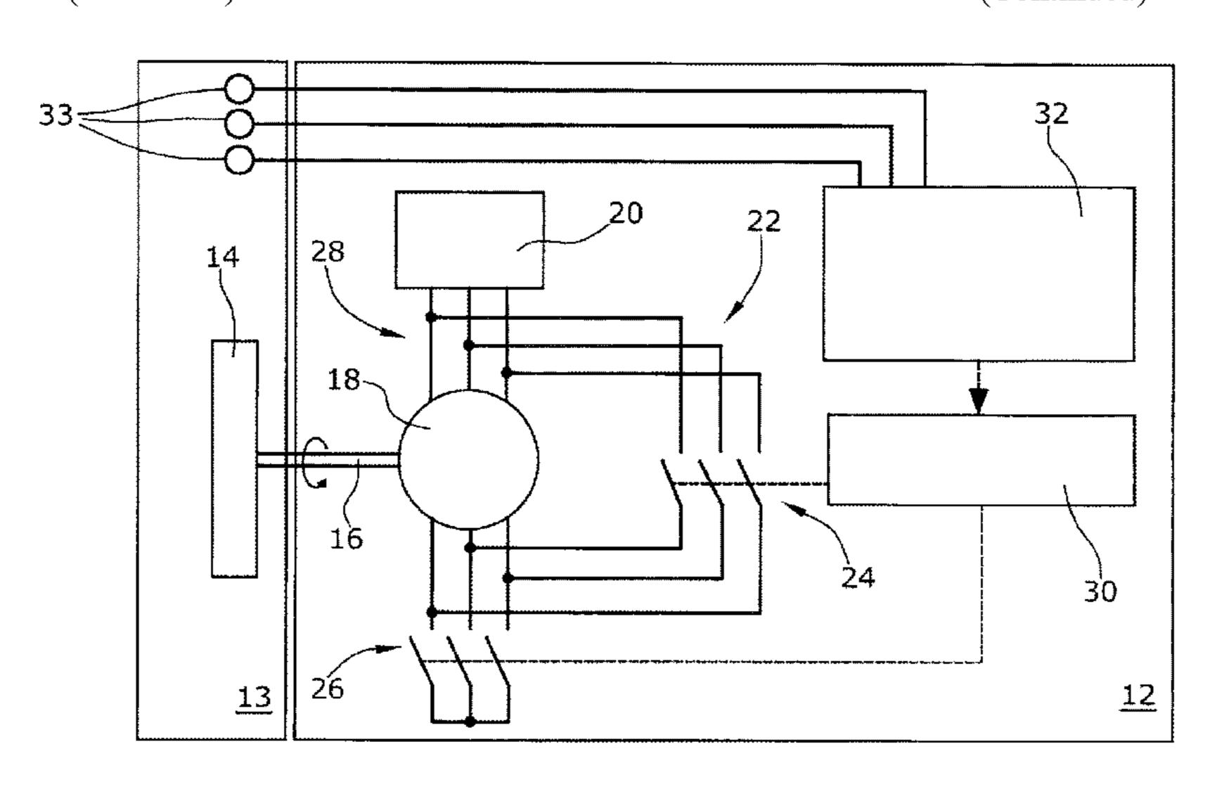
which is electrically or optically connected to the switchover device and the measuring device and which is designed to actuate the at least one switch on the basis of the measured value of the operating variable of the vacuum pump in order to produce the star-delta switchover.
