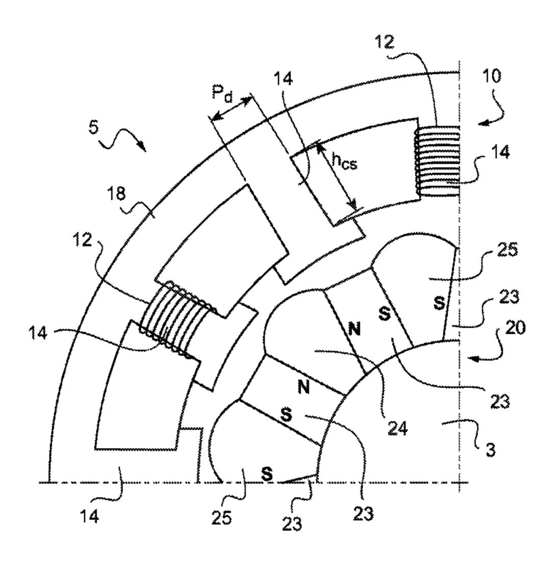
electromechanical conversion member is a flux-concentrating member and each winding is concentric and has a single layer. The electromechanical actuator is intended in particularly for controlling a hydraulic actuator via a mechanical transmission within an electrical flight control device of an aircraft.
