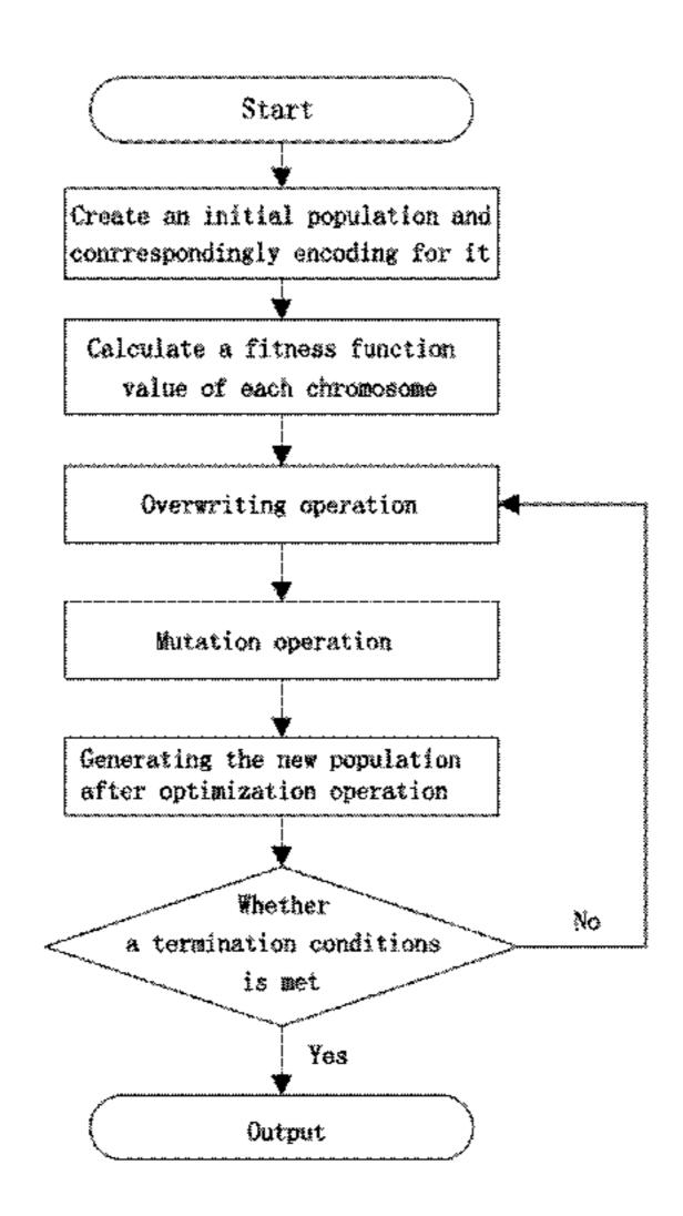
termined termination condition is met, and obtains the optimal population gene; then determines the array elements arrangement of the L-shaped array antenna according to the optimal population gene.
