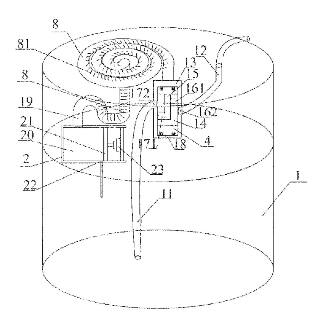
end of the liquid-reservoir space; the volume of the maximum sealing portion of the cylinder is greater than the volume of the liquid-reservoir space; the liquid-drawing channel communicates with the liquid-reservoir space; the outflow channel communicates with a tail end of the liquid-reservoir space.
