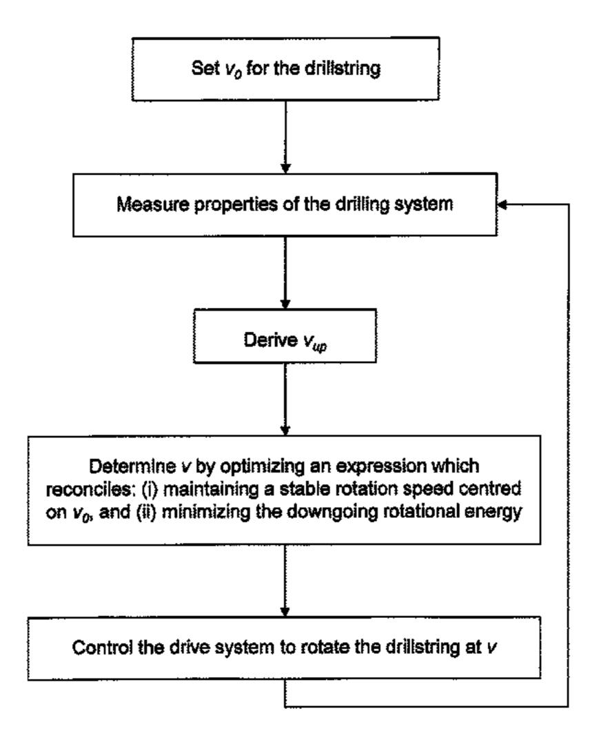
ematical expression containing a sum of downgoing rotational energy produced by the drive system and downgoing rotational energy caused by the upgoing rotational waves that are reflected downwardly at an upper end of the drill-string, and then optimizing the mathematical expression, which is then used for controlling the drive system to rotate the drillstring at v.
