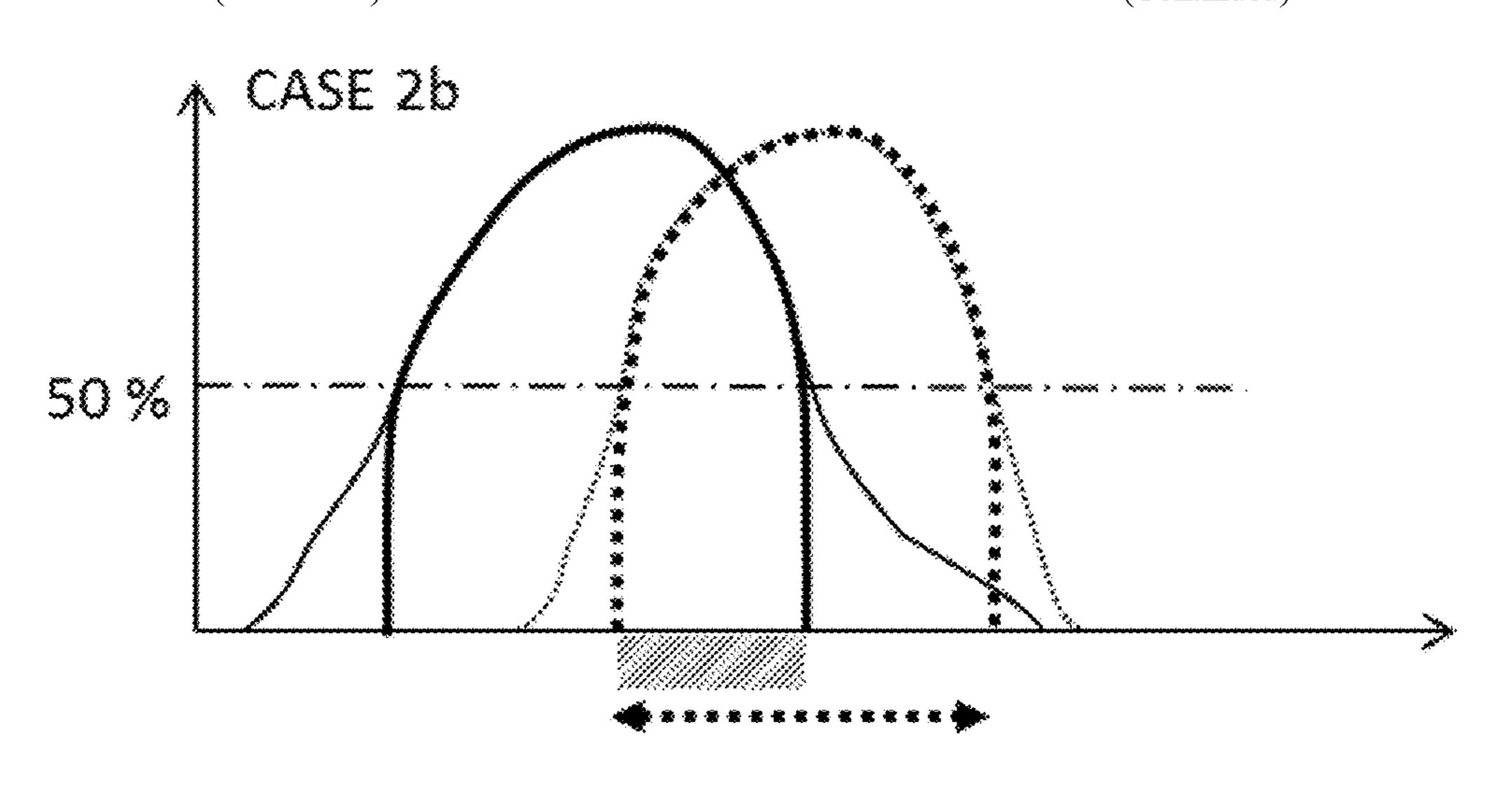
ond emission wavelength range, said first emission wavelength range overlapping with the excitation wavelength range of the second luminescent dye, so that upon irradiation within the excitation wavelength range of the first luminescent dye the second luminescent dye is excited, in the overlapping area of the patterns, to emit electromagnetic radiation in the emission wavelength range.
