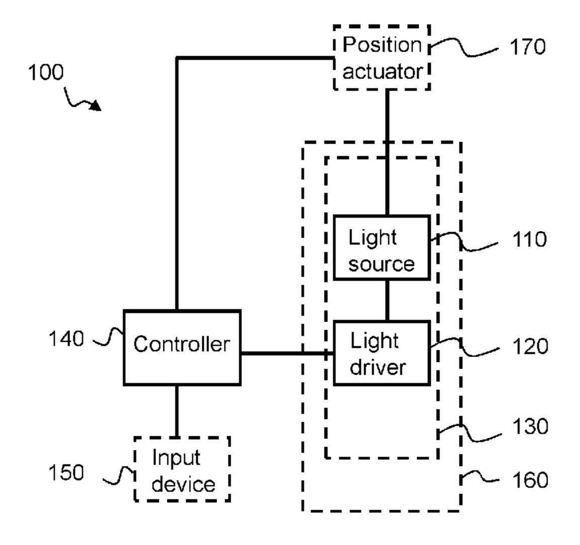
illumination system also comprises a controller (140) that is adapted to provide control signals to the light driver to increase a light intensity level of the light emitted from the at least one light source from a first light intensity level (II) to a second light intensity level (12) over a time period (T) of at least one day to two weeks, preferably at least two days to two weeks.
