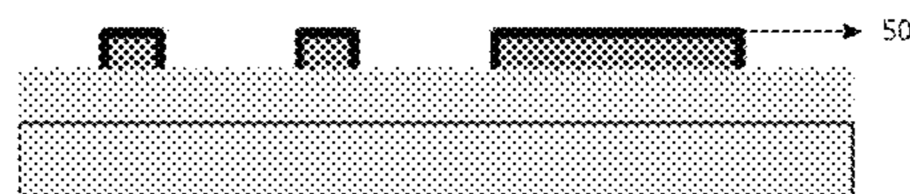
3) Embedding metal foil pattern into adhesive layer
