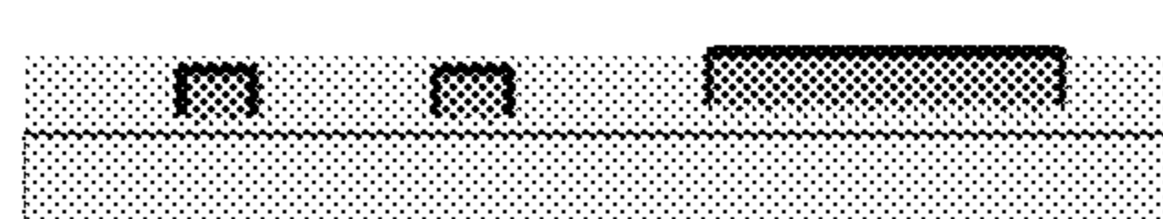
4) Removing blackening layer provided on upper surface of second metal foil pattern
