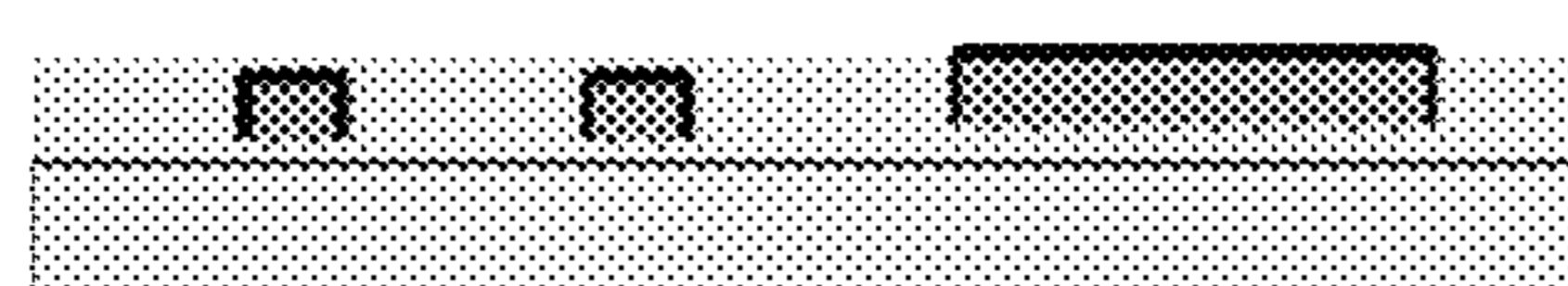
4) Removing blackening layer provided on upper surface of second metal foil pattern
