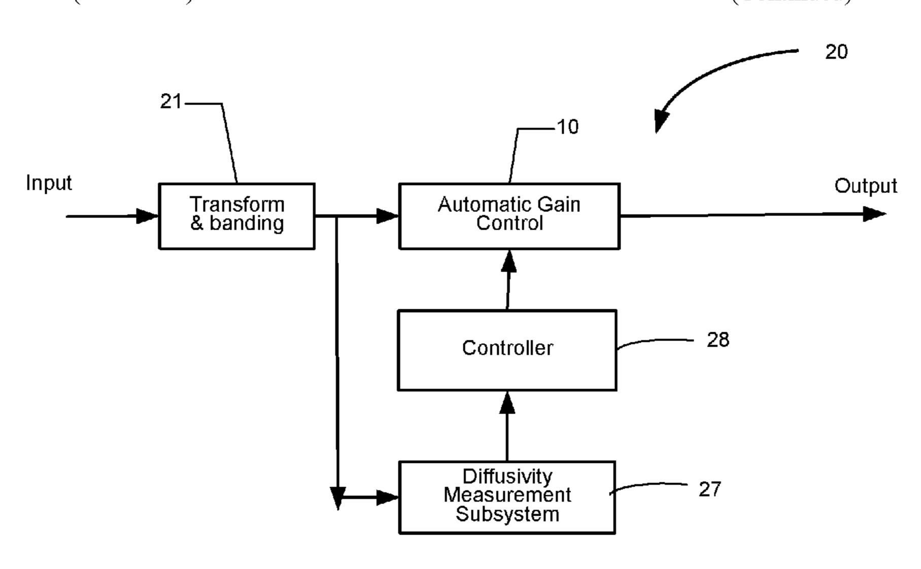
in the audio signal levels. A controller is operably coupled to the diffusivity measurement unit and the leveler unit to control the gain applied to the audio signals by the leveler unit based on the level of diffusivity of the sounds present therein.
