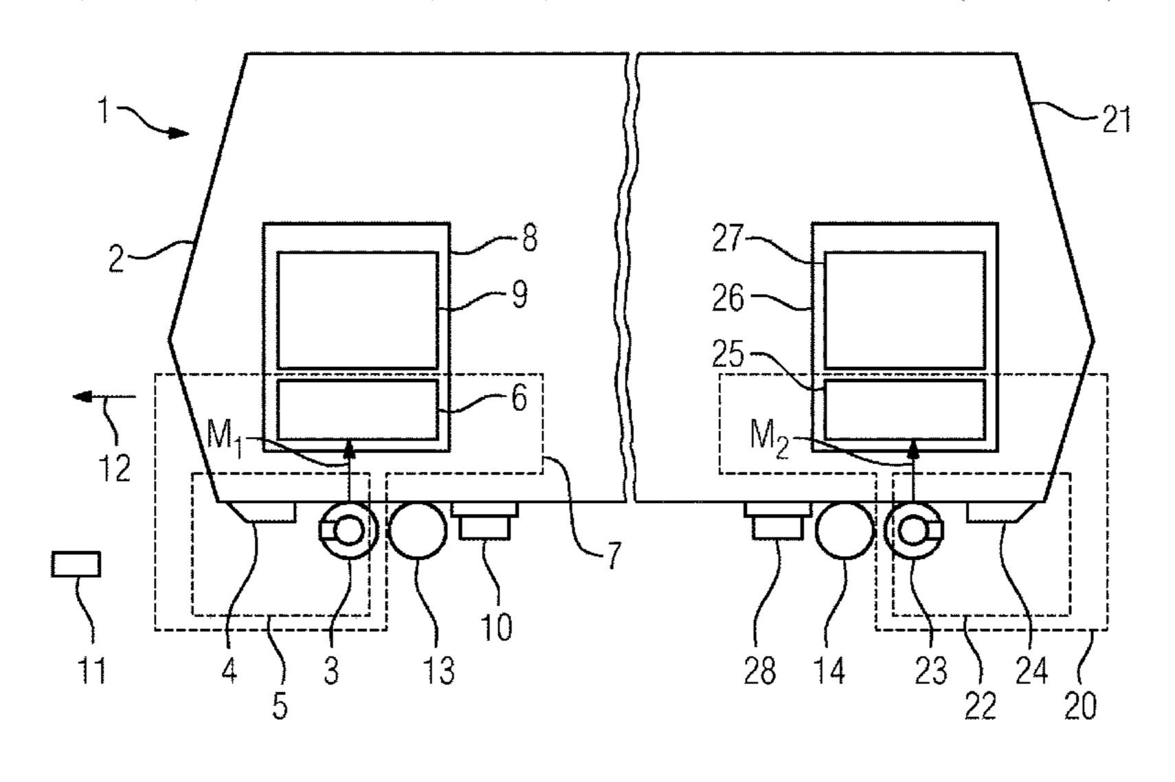
relative to the first position marker information recorder in the longitudinal direction of the vehicle and a generation of further position-determining distance measurement values is initiated. A positioning device for determining the position of a track-guided vehicle is also provided.
