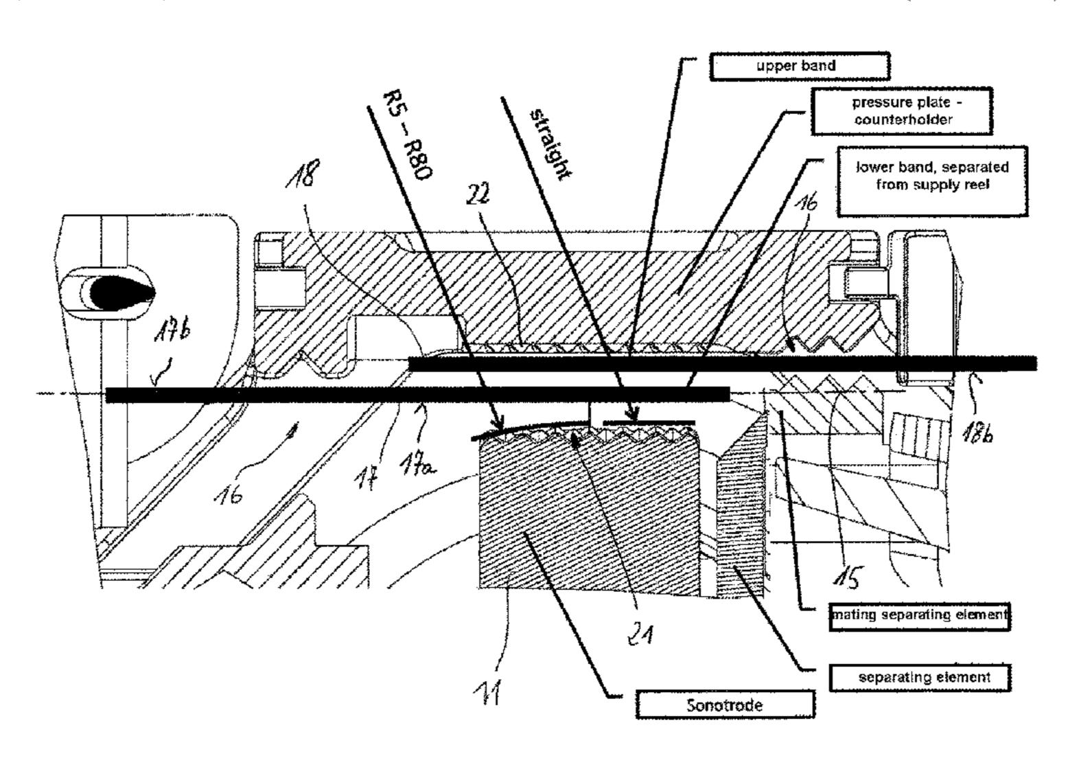
strapping devices. This is achieved in that the contact surface (21, 24) of the sonotrode (11) is aligned at an angle  $\alpha$  which deviates from a right angle relative to the provided vibration direction of the sonotrode (11).
