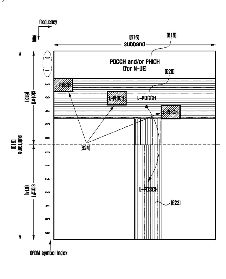
second type terminals. The L-MIB includes control information on an L-subframe configuration for supporting a second type terminal and a sub-band configuration of the L-subframe, while the L-SIB includes information on downlink reception and uplink transmission of the second type terminal. When the base station receives a Random Access Channel (RACH) preamble request from one of the terminals, the base station performs the random access procedure.
