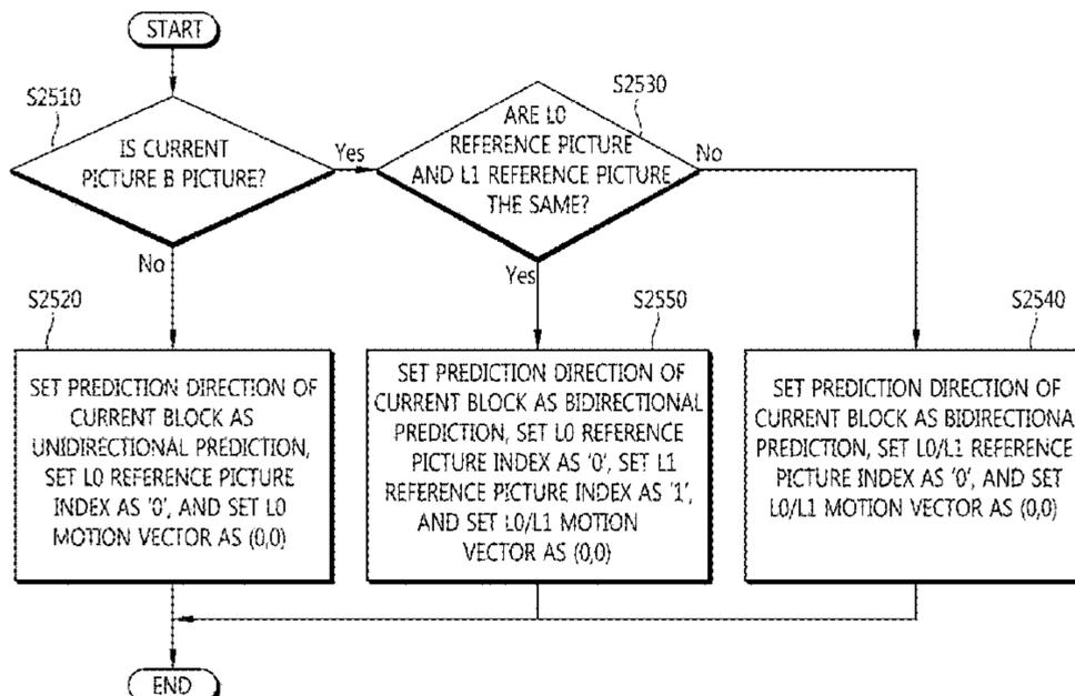
a current block; and generating a prediction block for the current block on the basis of the derived motion information. According to the present invention, computational complexity can be reduced and encoding efficiency can be improved.
