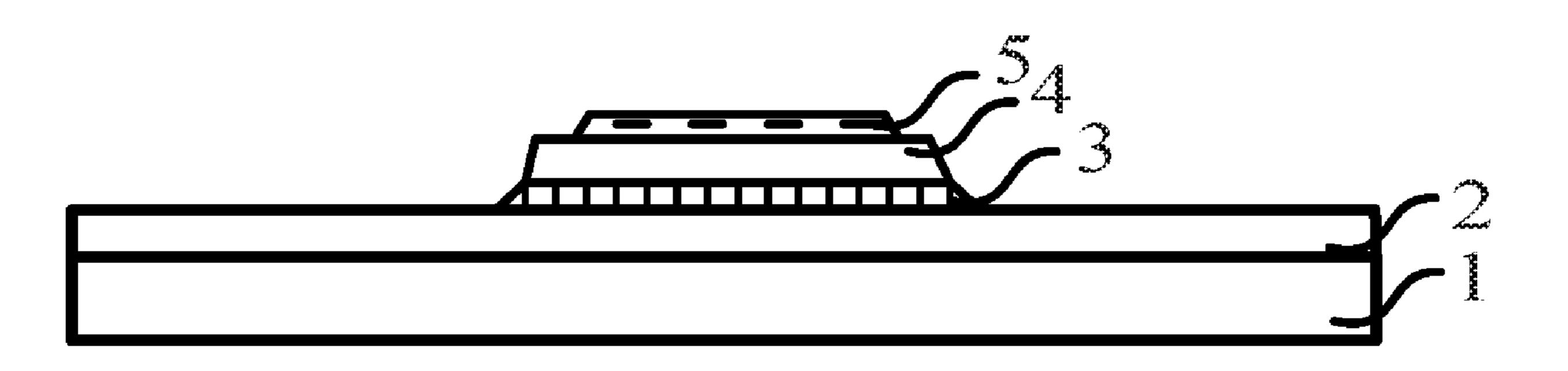
element as the light shielding layer of the LTPS substrate, which not only ensures the light shielding efficiency but also reduces the production process, and further prevents the occurrence of the H explosion problem due to H exuding during the ELA process.
