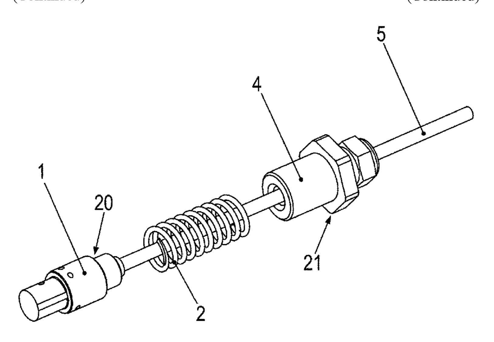
sensor housing is pressed against a step of the bore, in particular by the spring part.
