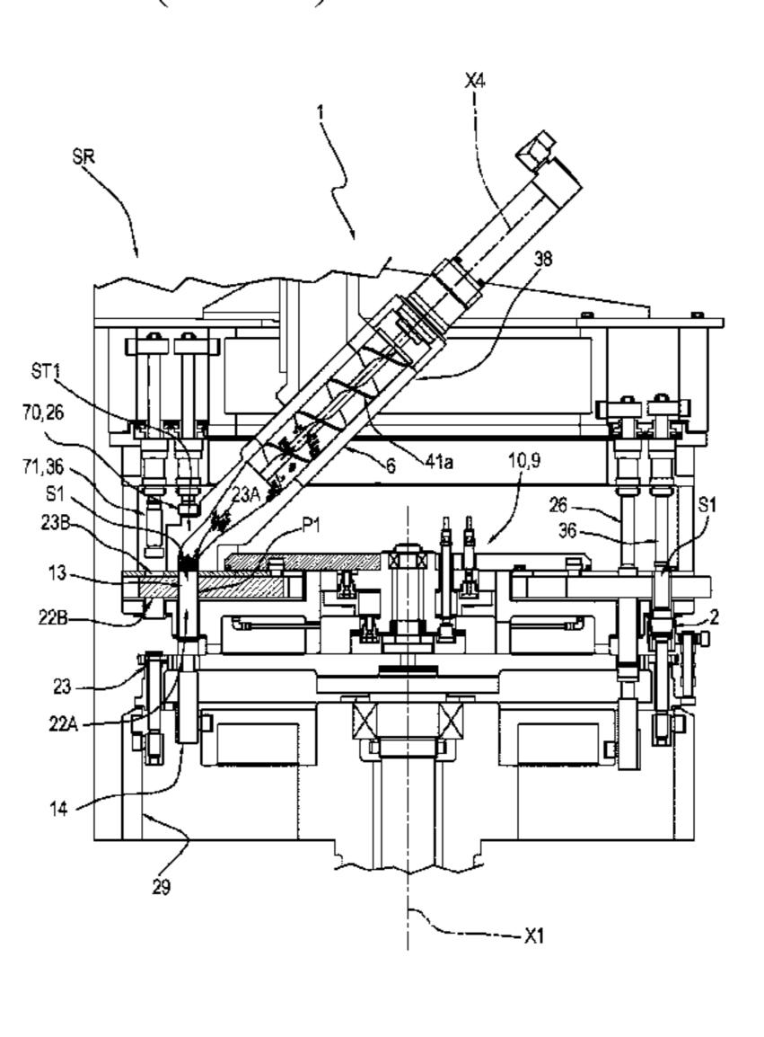
being configured for controlling the compacting device (70) with a force such as to produce a compression which causes a coupling of the dose (33) with the side walls of the containing seat (S1) which prevents, in the operating condition of the unit, the escape of the dose from the containing seat (S1) in the absence of actions mechanical for pushing on the dose.
