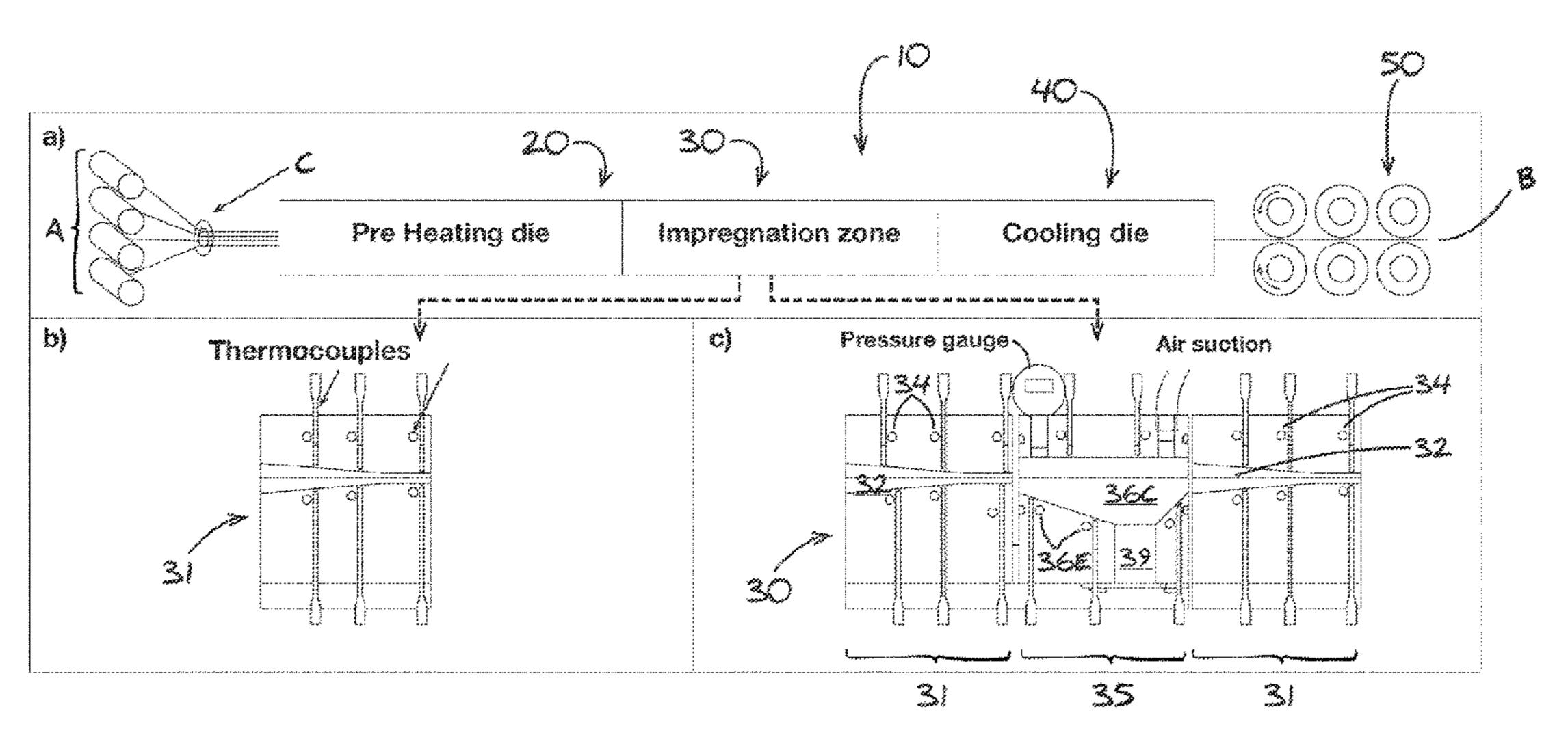
cool the beam before the beam reaches the pulling mechanism. A system for pultruding beams is also provided.
