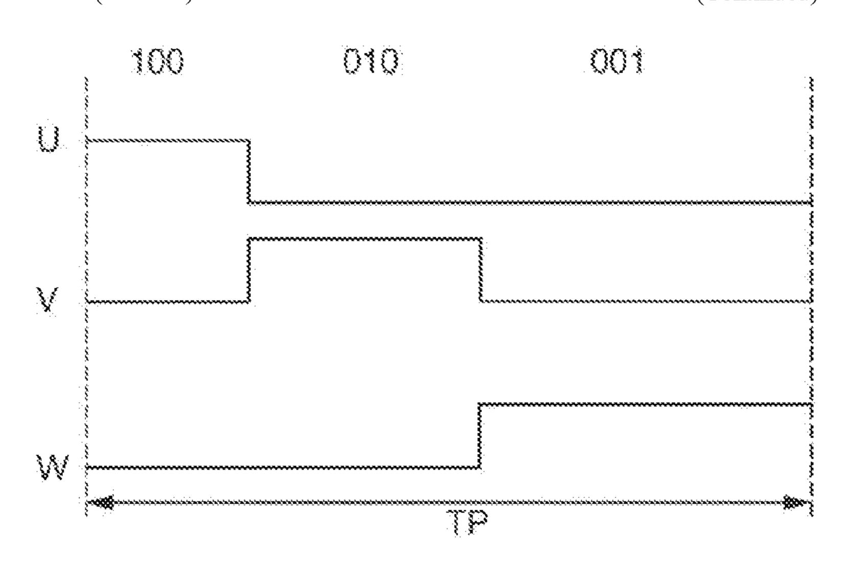
activated, wherein specific star point voltages ensue for various groups of switching patterns; and in at least one operating state of the frequency converter, within a respective period of the pulse width modulation, activating only those switching patterns in which an identical star point voltage ensues.
