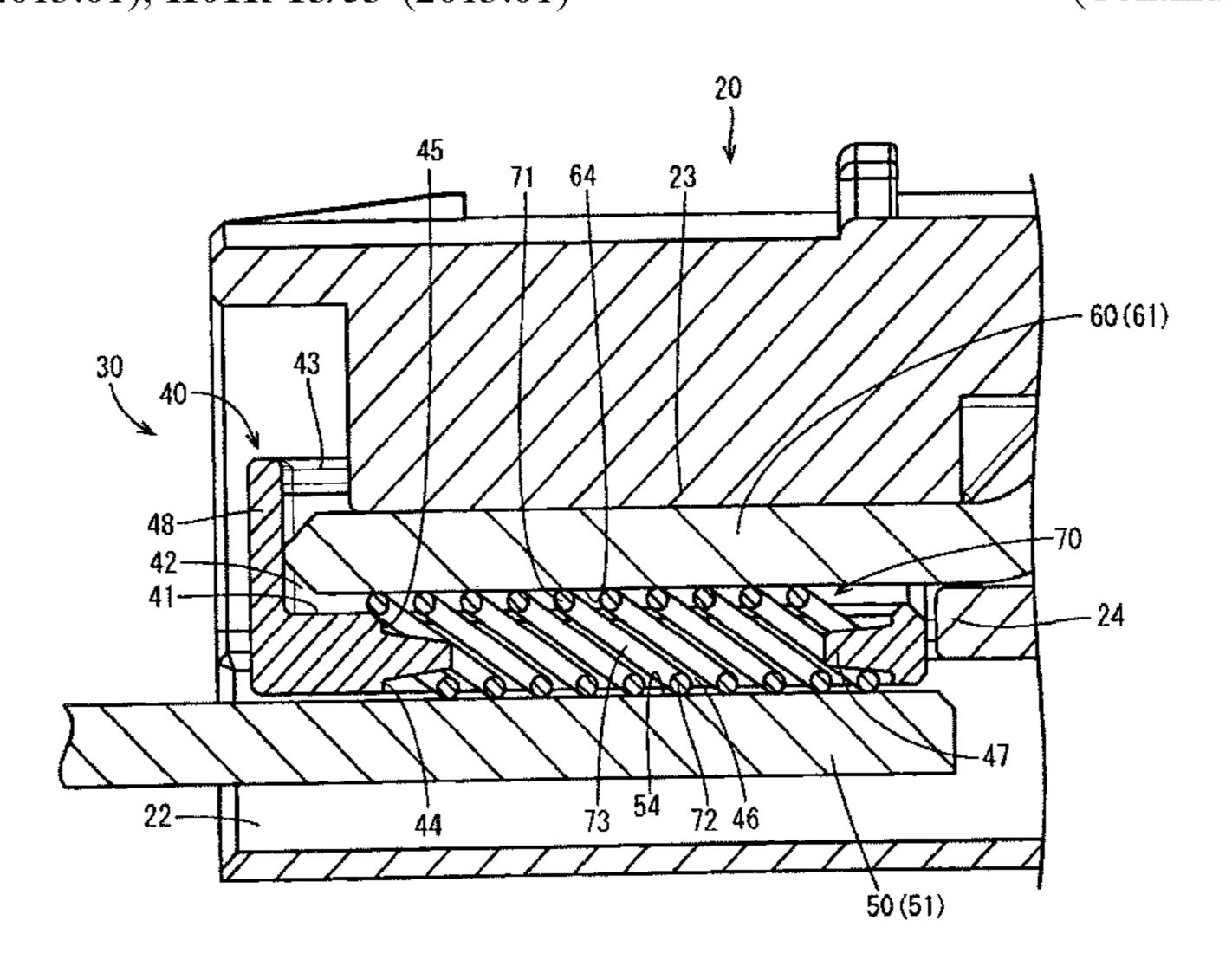
opening (45) approaches the female-side contact surface (64) as the coil spring (70) is compressed.
