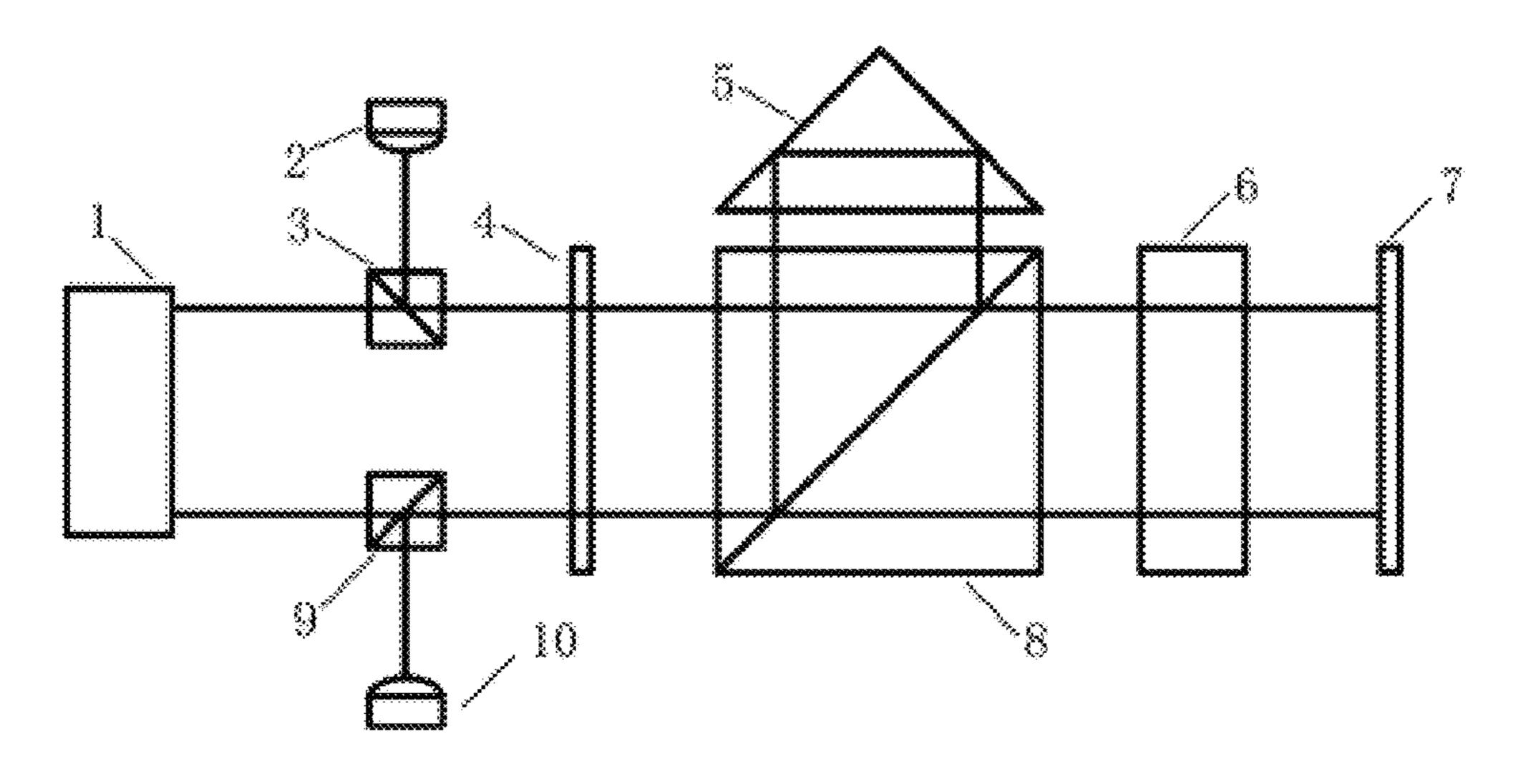
erodyne interferometry, simplifies the optical path structure, and improves accuracy of laser heterodyne interferometry.
