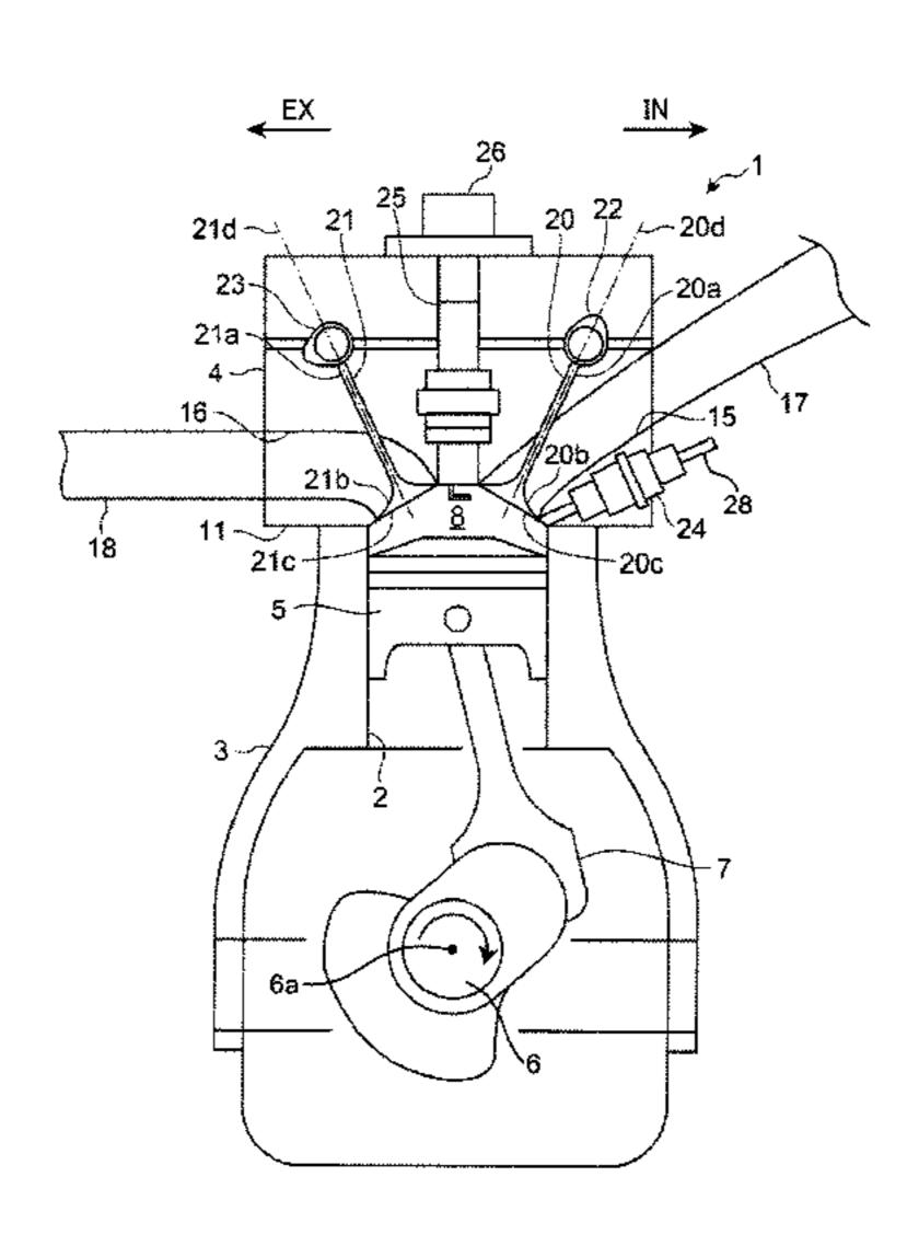
way that a ratio of a length of the exhaust-side inclined surface with respect to a length of the intake-side inclined surface is 1.25 or larger in a cross section passing through a center axis of the piston and orthogonal to an axis direction of a crankshaft.
