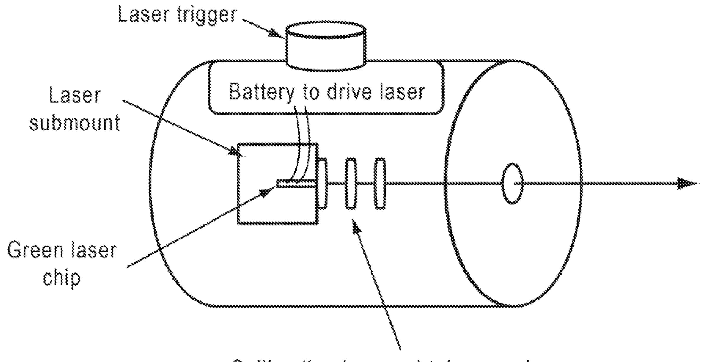
Collimation lens and telescope lenses to collimate and resize the beam
