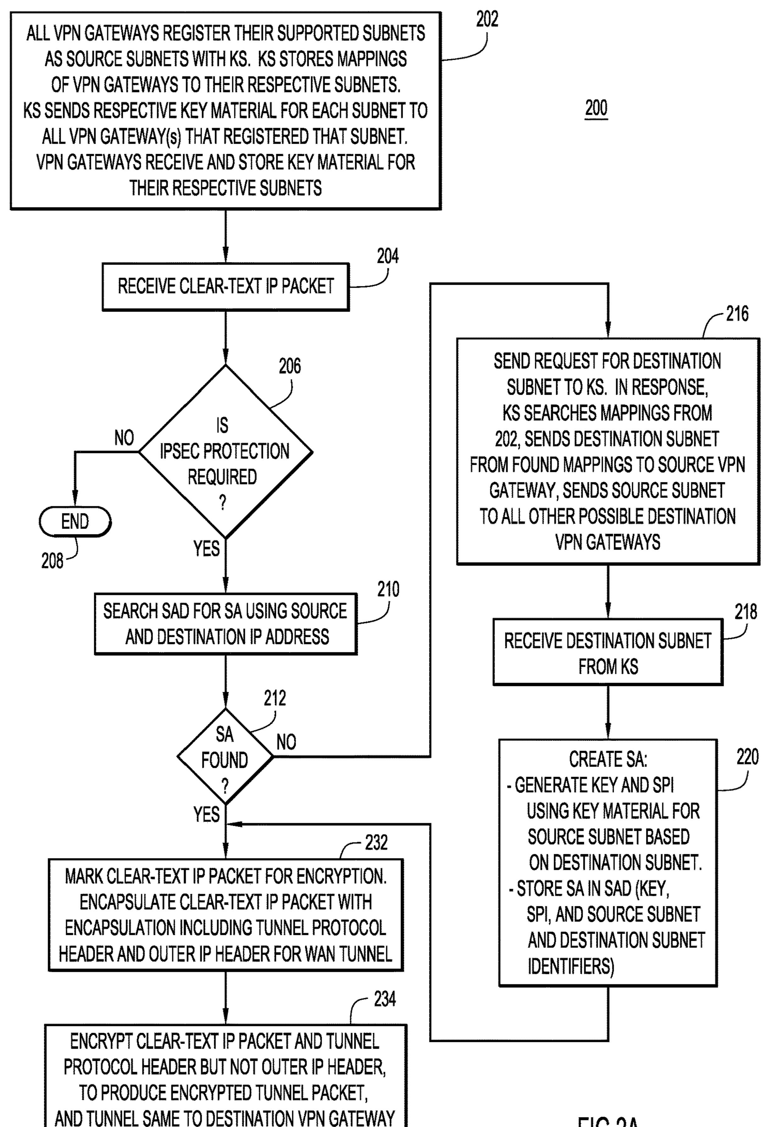
VPN GATEWAY BASED ON OUTER IP HEADER
