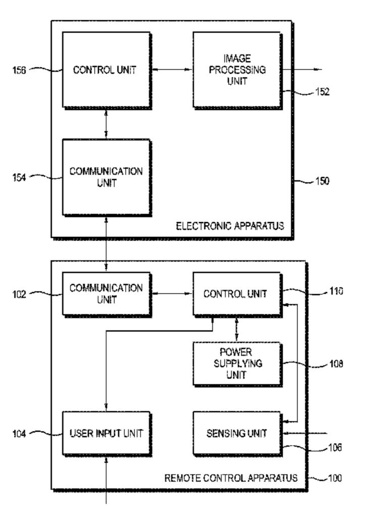
to perform a function corresponding to the input button if the remote control apparatus is in a button input mode, and to transmit information about the movement of the remote control apparatus to the electronic apparatus to control the electronic apparatus by the movement if the remote control apparatus is in a motion recognition mode. Accordingly, controlling a game or a multimedia content is easier, and the user is provided with a new and interesting experience.
