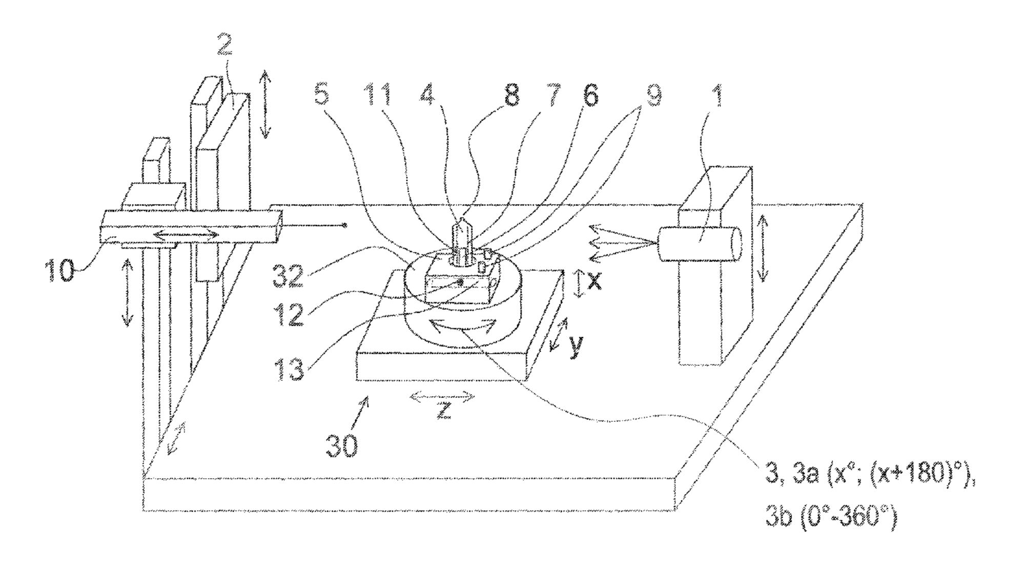
geometry feature by using any target geometry, in particular without the availability of a CAD model being necessary, according to the invention, in order to determine the geometry features, surface measurement points are used which are associated with the geometry features to be determined on the basis of specifiable rules and the geometry features are determined from the associated surface measurement points.
