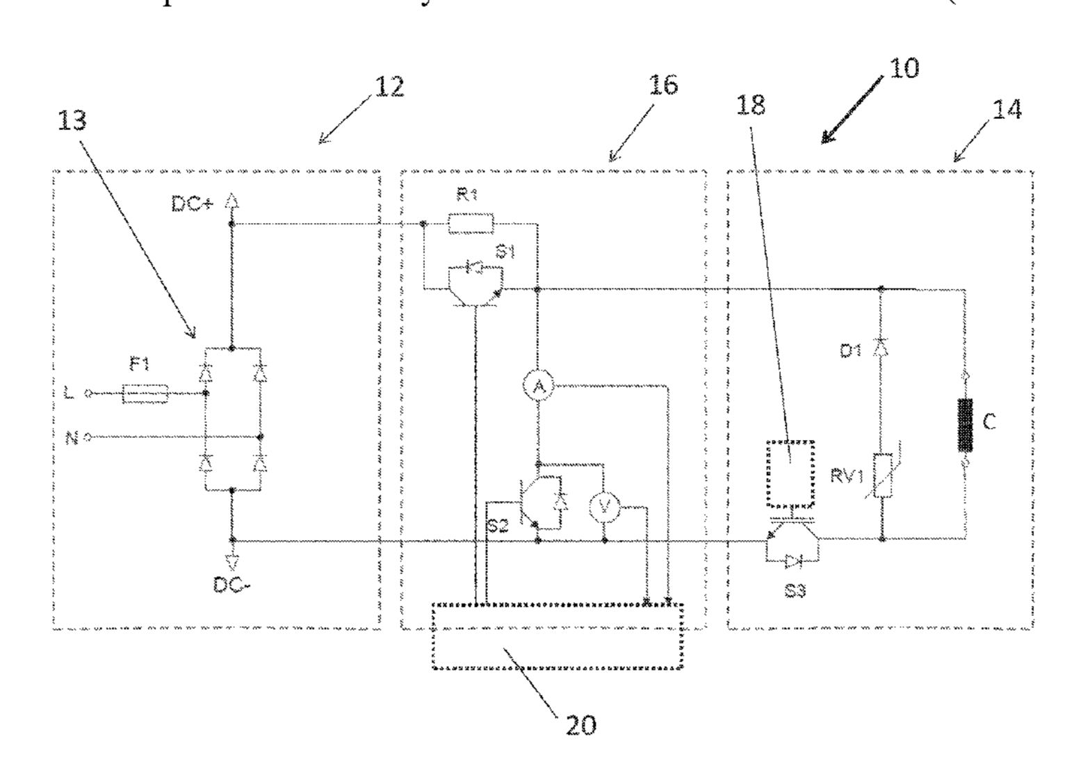
elevator safety circuit. This brake controller offers an improved cut-off safety in safety relevant situations.
