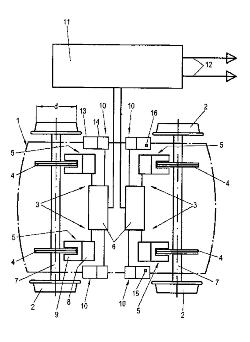
that, when a predetermined application force is actuated during braking operation, a value of the current wheel diameter detected by the determination unit is taken into account.
