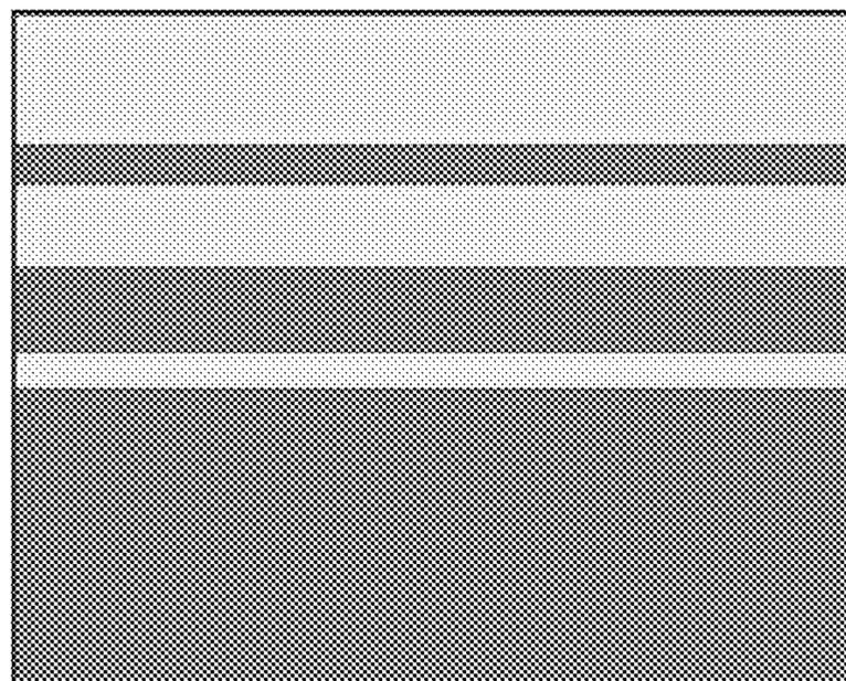
COMP-B and COMP-E are arranged in alternating order, and wherein the thickness of the individual layers B, Bx is decreasing from bottom to top and the thickness of the individual layers E, Ex is decreasing from top to bottom. The dental mill blank can be used for producing dental articles.
