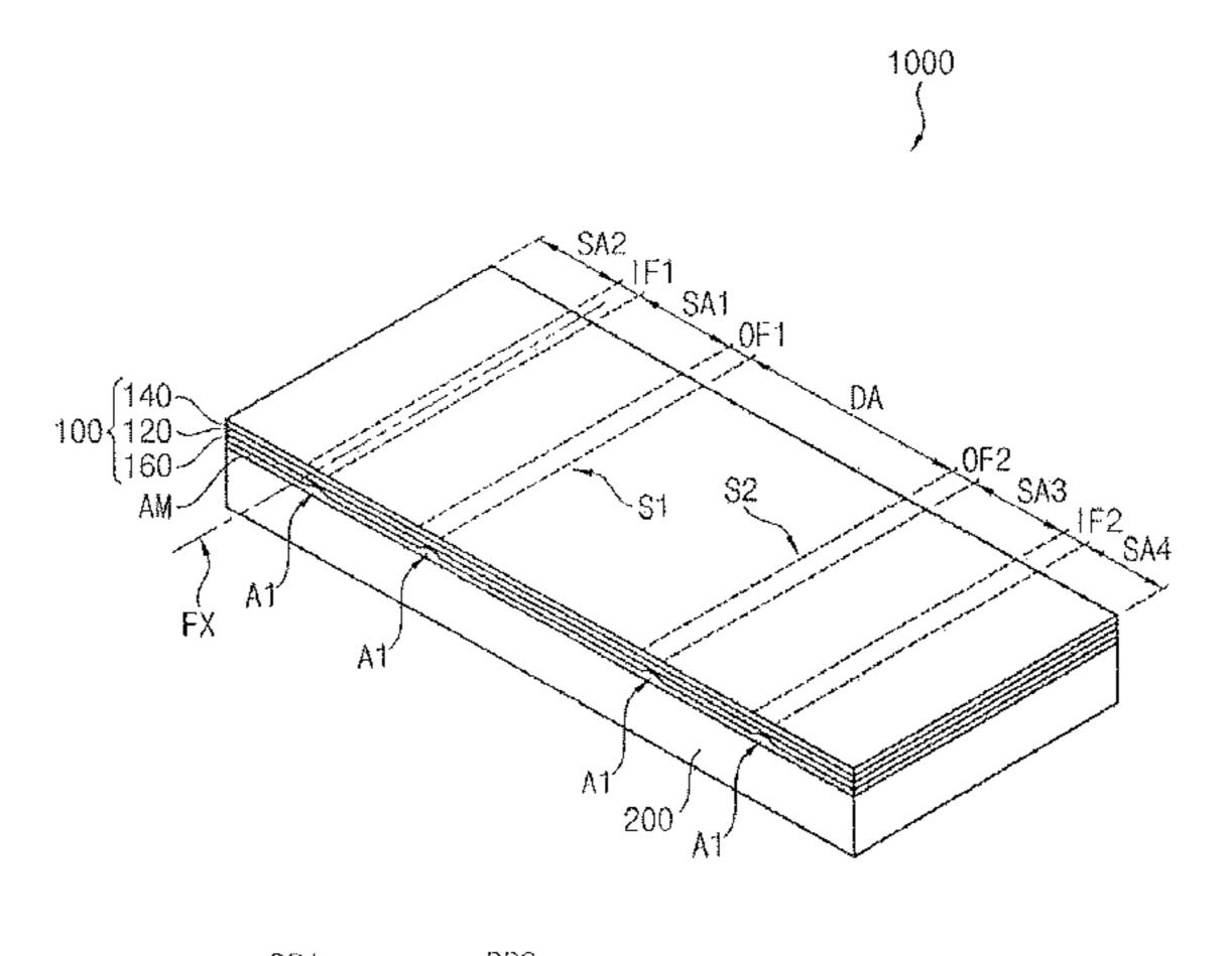
thickness of the first hard coating layer. A thickness of a first area of the second hard coating layer that overlaps with the out-folding area and the in-folding area of the base substrate is less than a thickness of a second area of the second hard coating layer that overlaps with the peripheral areas of the base substrate.
