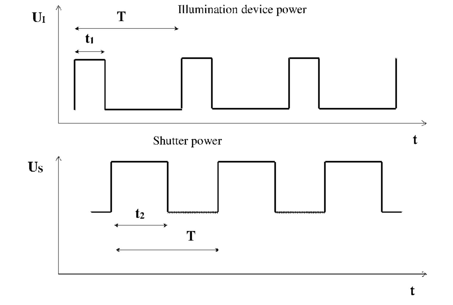
directed to a light-sensitive matrix of an astronomical instrument during arrival of the light flow pulses of the outdoor illumination devices. Thus, light pollution of astronomical instruments by outdoor illumination devices is avoided.
